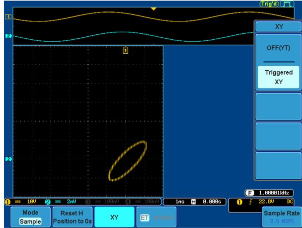
To move the X Y waveform position, use the vertical position knob: Channel 1 knob moves the X Y waveform horizontally, Channel 2 knob moves the X Y waveform vertically. Similarly, the X2 and Y2 axis can be positioned using the channel 3 and channel 4 vertical position knobs.
