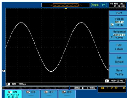
Vertical Navigation      Press *Vertical* repeatedly from the side menu to choose to edit the vertical position or Volts/Div. Use the Variable knob to edit the values.
