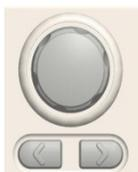
Scroll wheel is used to set each parameter value, whilst arrow keys are used for parameter, menu selection and voltage/current fine adjustment. It is used to switch or operate the displayed waveforms under diagram display mode.
