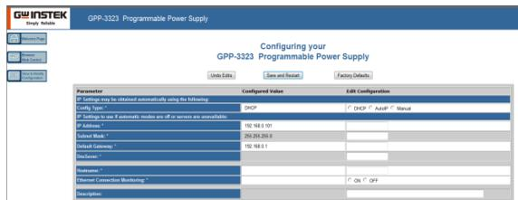
4. Click “Modify Config” to enter the network configuration setting menu, as shown below. Use the mouse to click on “Save and Restart” to change the remote settings for the GPP series.
