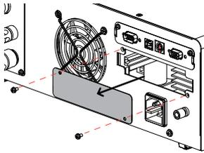
2. Insert the GPIB card into the opening of rear panel. Push the card gently until it is fully inserted followed by fastening the screws.
