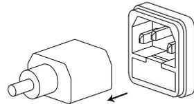
3. Remove the fuse socket using a flat screwdriver.
