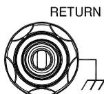
The RETURN terminal is used for ACW, DCW, IR and CONT tests.
