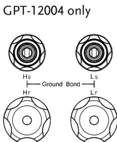
The SENSE H, SENSE L, SOURCE H and SOURCE L, terminals are used for GB (Ground Bond) test.
