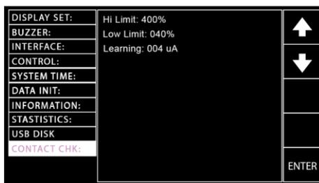
3. Press the ENTER soft-key to enter the Hi Limit setting followed by using scroll wheel to determine an exact scale of Hi Limit threshold that triggers the SHORT status warning.
