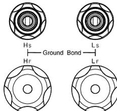
The SENSE H, SENSE L, SOURCE H and SOURCE L, terminals are used for GB (Ground Bond) test.
