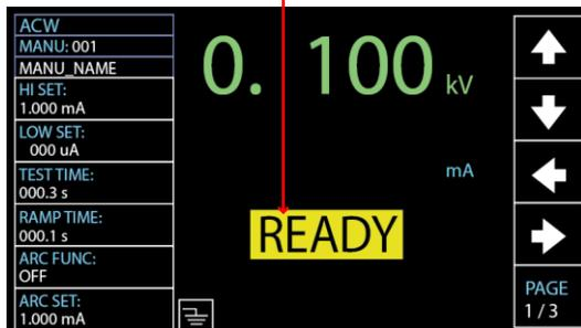
2. Press the START button when the tester is in the READY status. The manual test starts accordingly and the tester goes into the TEST status.
