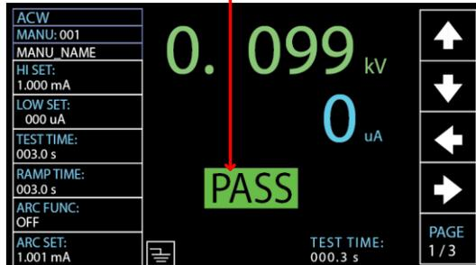
2. The tester will immediately restore back to the READY status after PASS judgment. However, if the PASS HOLD is activated, PASS judgment will persist until the set duration of PASS HOLD is fully met. Refer to page 63 for details.
