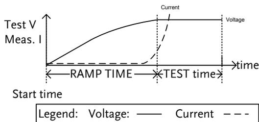
The test items that are plotted on the sweep graph depend on the type of test that is performed.
