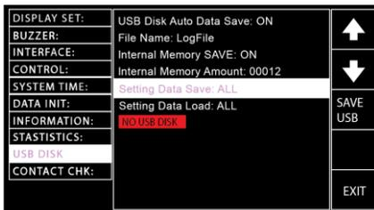
8. Press the UP/DOWN arrow soft-keys to move the cursor to the Setting Data Load setting, which allows user to load individual data including MANUDATA, AUTODATA and SYSDATA or All data from the USB disk.
