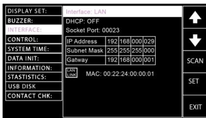
When pressing the SCAN soft-key, the unit will scan the LAN card setting thoroughly. In fact, the unit automatically scans at once every time when Interface is changed to LAN setting.
