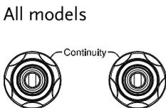
The OUTPUT terminal (red) and RETURN terminal (black) are used for CONT (Continuity) test.
