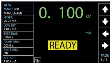
**AUTO Mode**      AUTO mode indicates that the tester is automatic, which consists of a sequential AUTO test of up to 10 MANU steps. Also, several groups of AUTO tests can be further interconnected for an advanced AUTO test.
