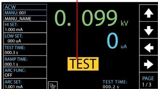
3. The test will start by showing the ongoing ramp up time followed by the ongoing test time and the ongoing ramp down time. The test will continue until the test is finished or stopped.
