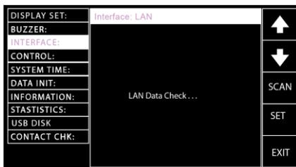
If LAN card with network setting is scanned properly, the “LAN LINK” icon appears. If not, however, the icon doesn’t appear.
