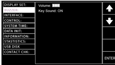
3. Press the ENTER soft-key to enter the Volume setting followed by using the scroll wheel to set the Volume level.
