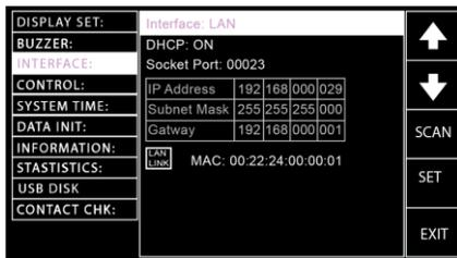
When LAN setting is scanned properly and Interface is set as LAN, the “LAN LINK” icon shows as the following figures.
