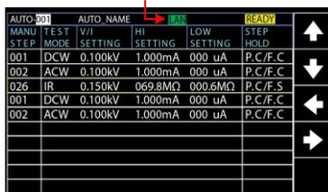
When LAN setting is Not scanned properly and Interface is set as LAN, the “LAN OPEN” icon shows as the following figures.
