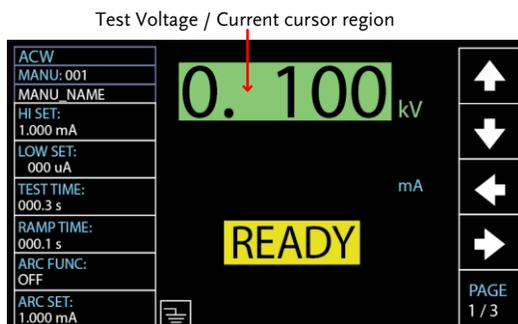
2. Use the scroll wheel to set the test voltage or ampere level.
