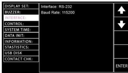
3. Press the ENTER soft-key to enter the Interface setting followed by using the scroll wheel to select the Interface options.
