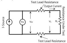
The figure below shows the 4-wire sense mode which add another set of test leads to connect the SENSE HI and LO terminals to the resistor under test on the basis of the 2-wire connection to minimize the effects of lead. Because of the high input impedance of the  $V_{\rm M}$  (voltmeter), the current of the sense leads connected to both ends of resistor under test can be ignored, and the voltage measured by the voltmeter is the voltage at both ends of the resistor under test.
