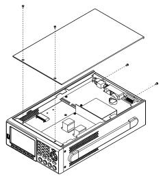
2. Move the top cover back slightly to release the buckle, and then lift the top cover up. Find the location indicated by the arrow in the figure shown below(close to the fan) and then replace the battery with a new one.
