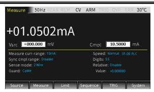
!WARNING: When the GSM is used as a voltmeter, Cmpl must be set to be higher than the voltage that is being measured. If this setting is not done, excessive current will flow into the GSM and cause damage.
