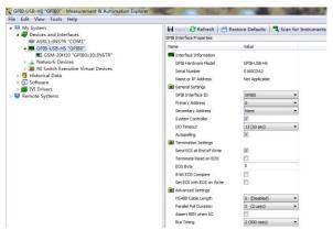
Click "Scan for Instruments" button to display the connected instrument information.
