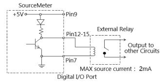
Sink current operation: connect an external relay between one of digital output lines and the +5V power supply. The digital output line must be set to low level to drive the relay. The maximum sink current is 500mA. The connection method is shown in the figure below:
