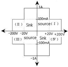
1A, 20V and 100mA, 200V amplitude is the nominal value. The actual maximum output voltage and output current amplitude are 1.05A, 21V and 105mA, 210V. The limit in the image above is not a range.
