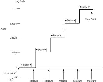
When starting sequence, the output will go from the bias level to the Start piont, and run to the Stop point in equal logarithmic steps. When the trigger delay time is set to 0, the time of each step is determined by the source delay time and the time it takes to perform measurement (NPLC setting).
