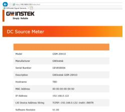
2. Click the "WEB CONTROL" to enter the network control interface, as shown in the figure below. Through the SCPI Command box, you can execute all Commands such as querying, setting information, measurment, and reading information. For example, input the "\*IDN?" query Command in the SCPI Command box,
