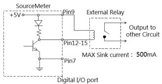
Output Enable control line The digital I/O port provides an output enable control line to be used together with the output switch of a test fixture. When used correctly, the Output of the GSM will turn off if the lid of the test fixture is opened.
