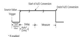
The delay of the SDM cycle can make the source stabilize before the measurement. The source delay can be manually set from 0000.00000 seconds to 9999.9990 seconds using Delay setting box; if the Auto delay is Enabled, the delay time depends on the presently selected source range.
