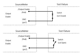
NOTE: The Output enable line can be driven by Digital I/O. Allow 100us settling and response time. The digital I/O lines are edge-sensitive, open-collector, and signals must be debounced to avoid unstable operation.
