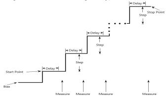
When starting sequence, the output will go from the bias level to the Start point, and run to the Stop point in equal steps. When the trigger delay time is set to 0, the time of each step is determined by the source delay time and the time it takes to perform measurement (NPLC setting).
