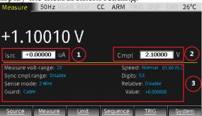
For example, to measure 1.05mA current, set the power supply as V-Source, set  $V_{\rm src}$  to 000.000mV, Cmpl to 10.5mA, and set Measure curr-range to 10mA. Press the output button to display the measurement reading.
