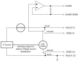
Source I When configured as an I-Source, the GSM operates as a high-impedance current source with voltage limiting capability and can measure current (as an ammeter) or voltage (as a voltmeter).
