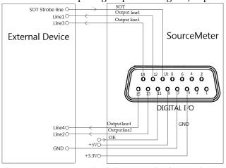
The measurement method shown in the figure above is used to send the pattern values of the limit test. Each open-collector output can be set to high level (+5V) or low level (0V), and can source 2mA current or sink 500mA current.
