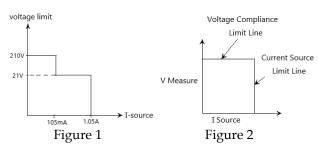
Figure 2 shows the limit line of I-Source, describe the maximum current limit value corresponding to the  $I_{\text{src}}$  range presently selected. For example, if it is on the 100mA current source range, the current source limit value is 105mA. The voltage compliance limit line represents the actual compliance value. The compliance value can be a real value or a range. These limit values represent the operating limits of the GSM in this quadrant. Restricted to any point in
