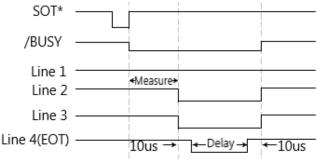
NOTE: When the trigger event in the trigger mode selects ↓STEST, the SOT signal is a falling edge trigger. When the trigger event in the trigger mode selects ↑STEST, the SOT signal is a rising edge trigger. When the trigger event in the trigger mode selects ↑↓STEST, the SOT signal is a rising or falling edge trigger.
