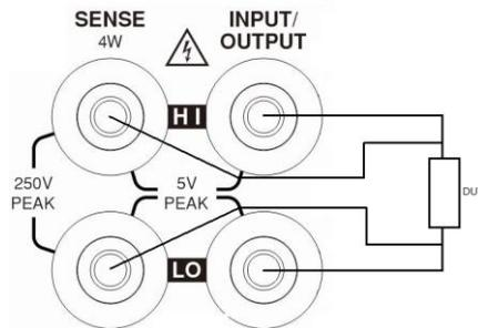
**!** **NOTE:** Specified accuracies for both source and measurement can only be achieved using 4-wire remote sensing.
