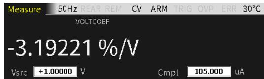
**VarAlpha**      Used to measure the varistor  $\alpha$  value.
