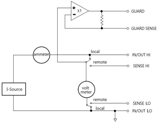
**⚠ NOTE: The current source does not require or use Sense leads to improve the accuracy of the current source. When selecting 4-wire sensing, the sensing leads must be connected, otherwise it will cause incorrect results. Please refer to page 35 for the connection method. If there is a possibility that the sensing lead may disconnect, overvoltage protection (OVP) can be used.**
