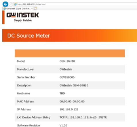
2, Click the "WEB CONTROL" to enter the network control interface, as shown in the figure below. Through the SCPI Command box, you can execute all Commands such as querying, setting information, measurement, and reading information. For example, input the “\*IDN?” query Command in the SCPI Command box,
