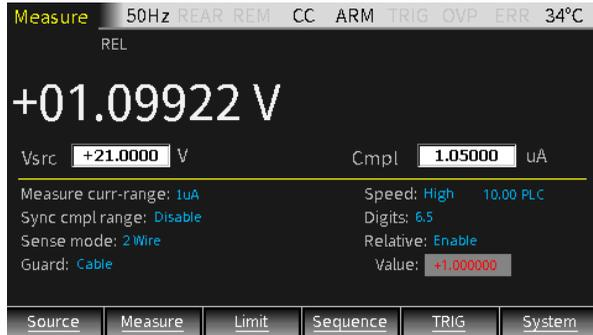
As shown in the figure below, connect a 20Ω resistor. When Isrc is set to 105mA, the output voltage should be 2.1V, Cmpl is set to 21V, and the output voltage is within the compliance value range. At this time, it is in CC mode. Relative option selects Enable, Value is set to 50mA, press the Output button. The displayed value is the difference between the output current value flowing through the load and the Relative Value.
