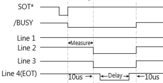
**⚠️ NOTE:** When the trigger event in the trigger mode selects ↓STEST, the SOT signal is a falling edge trigger. When the trigger event in the trigger mode selects ↑STEST, the SOT signal is a rising edge trigger. When the trigger event in the trigger mode selects ↑↓STEST, the SOT signal is a rising or falling edge trigger.
