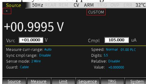
**NOTE:** When Counts option is set to Infinite, that is, when the times of sequence is infinite, the \* symbol will not appear on the upper left of the interface.
