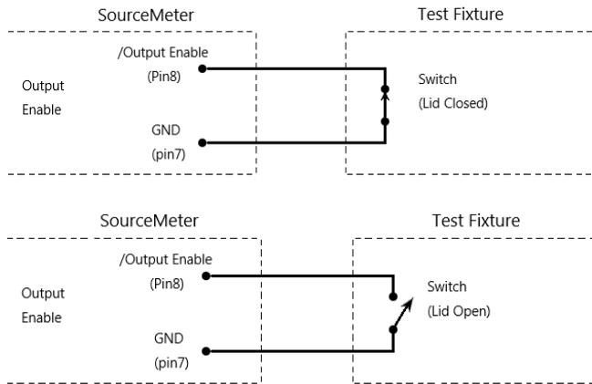
**⚠ NOTE: The Output enable line can be driven by Digital I/O. Allow 100us settling and response time. The digital I/O lines are edge-sensitive, open-collector, and signals must be debounced to avoid unstable operation.**
