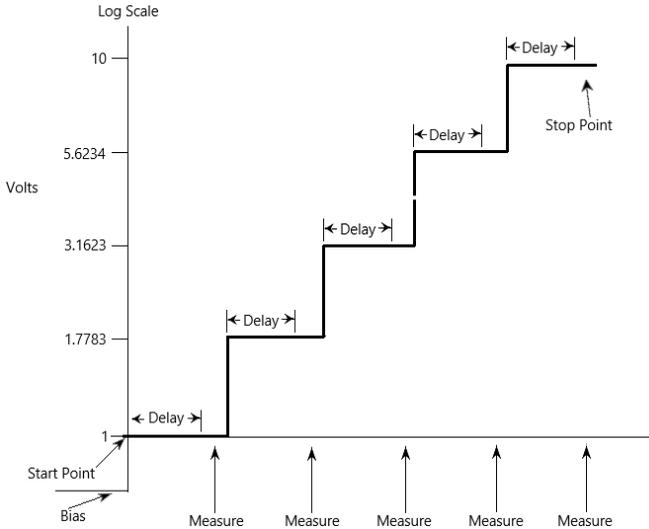
When starting sequence, the output will go from the bias level to the Start point, and run to the Stop point in equal logarithmic steps. When the trigger delay time is set to 0, the time of each step is determined by the source delay time and the time it takes to perform measurement (NPLC setting).
