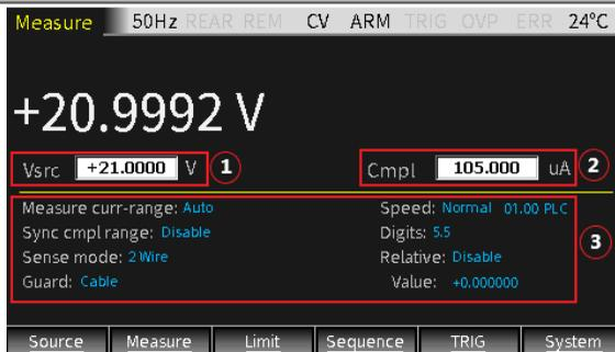
1. The Measure interface is basically the same as the Source (only increase setting items for resistor measurement). The parameter setting area is composed of 3 areas shown as ①②③ in Figure above. Press the Edit/Lock key to switch between ①②③.
