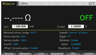
**Description** Use  $I_{src}/V_{src}$  to set the source value when measuring resistor.
