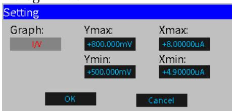
There are 4 choices of Graph: I/V, V/I, V/t, I/t; Xmax, Xmin, Ymax, Ymin are the maximum or minimum coordinates value of the X and Y axes. (NOTE: It is better to set the coordinates of data graphics with the full screen display)
