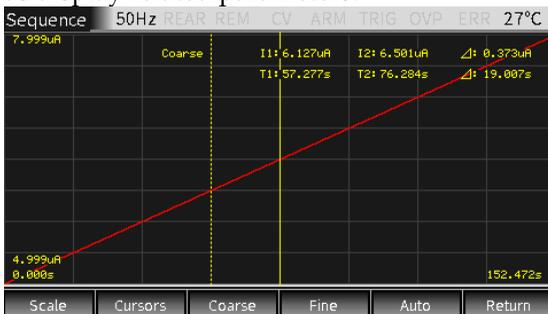
Cursors key has loop function, followed by "cursor and parameters display, cursor 1" → "cursor 2" → "cursors and parameters disappear"... (NOTE: the dotted line cursor is in the selected state)
