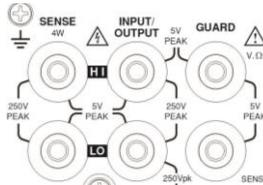
There are six terminals, including two power Input and Output positive and negative terminals, two voltage feedback positive and negative terminals, one guard terminal and one guard sense terminal. Please refer to the printing of the back panel for the specific order. See page 27 for details.
