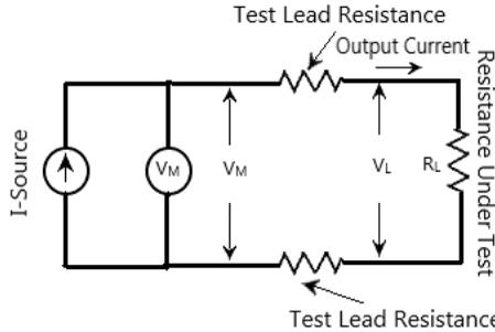
The figure below shows the 4-wire sense mode which add another set of test leads to connect the SENSE HI and LO terminals to the resistor under test on the basis of the 2-wire connection to minimize the effects of lead. Because of the high input impedance of the  $V_M$  (voltmeter), the current of the sense leads connected to both ends of resistor under test can be ignored, and the voltage measured by the voltmeter is the voltage at both ends of the resistor under test.
