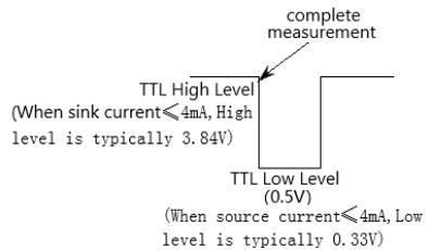
Output trigger provides a TTL compatible pulse level that can be used to trigger other peripherals.
