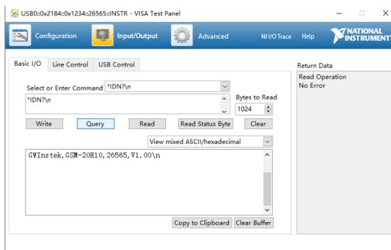
Enter the query Command “\*IDN?” as shown above, and the instrument identification information such as manufacturer, model, serial number and software version will be returned. The message "Read Operation No Error" is displayed in the Return Data window.
