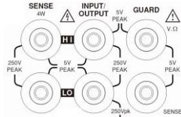
**! WARNING: To prevent electric shock and damages to the GSM-20H10, DO NOT exceed the maximum allowable voltage differentials shown in terminals. The front and rear terminals of the GSM are rated for connection to circuits rated Installation Category I only. Do not connect the GSM terminals to CAT II, CAT III, or CAT IV circuits. Connections of the GSM Input/Output terminals to circuits higher than CAT I can cause damage to the equipment or expose the operator to hazardous voltages.**
