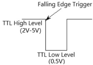
Input trigger is falling edge trigger, TTL compatible pulse level.
