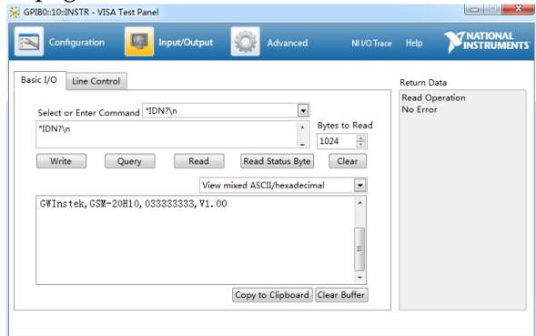
Enter the query Command “\*IDN?” as shown above, and the instrument identification information such as manufacturer, model, serial number and software version will be returned.
