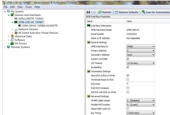
Click “Scan for Instruments” button to display the connected instrument information.
