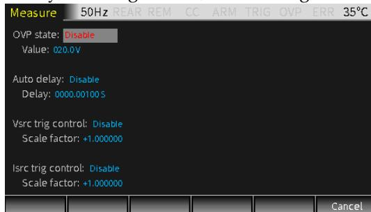
**OVP** Press the up and down arrow keys to move the cursor to the OVP state option box and press the Enter key to select Enable or Disable.
