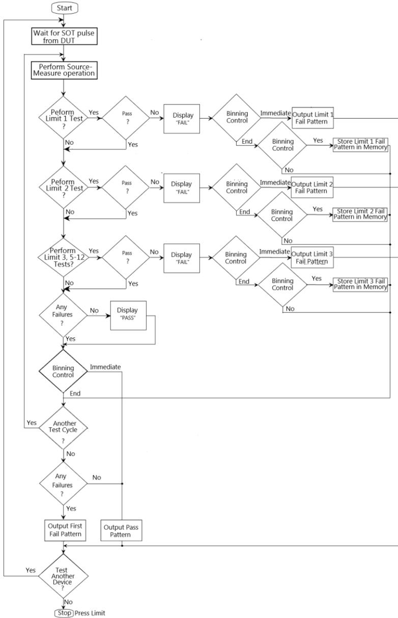
**SORTING mode:** If a measurement reading fails the Compliance Test, or is not within any SW-Limits range, the Limit test will display FAIL. If the measurement reading passes the Compliance Test and only Limit 1 is enabled, the corresponding Pass pattern value will be output. If in addition to Limit 1, SW-Limits also has an item that is Enabled, in the case of Limit test PASS, the I/O port outputs the Lo\_fail value of the first limit test band that passes (Hi\_fail value is ignored).
