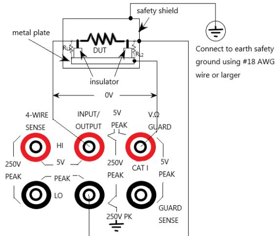
**Ohms guard:** Provide low internal resistor ( $<1\Omega$ ), high output current (up to 50mA) drive protection, allowing resistor measurement in the circuit. When measuring the resistor component in the resistor network, eliminate the influence of the resistor in parallel with it.
