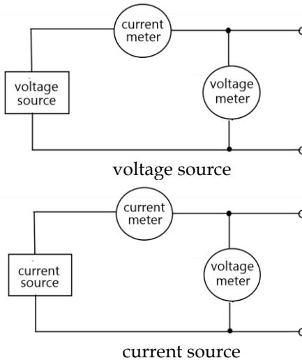
**Source V** When configured as a V-Source, it operates as a low-impedance voltage source with current limiting capability and can measure current (as an Ammeter) or voltage (as a voltmeter).
