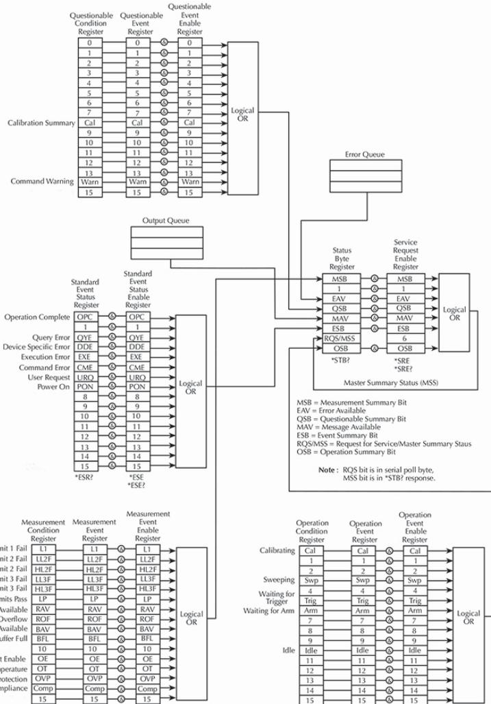
**! NOTE:** URQ indicates that the "Lock" key on the panel has been used. (Entering lock from unlock or Entering unlock from lock).
