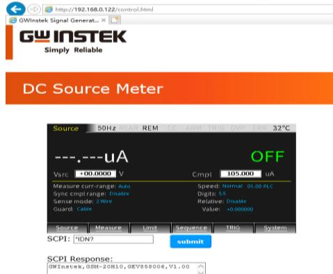
3、Click the "WEB CONFIG" to enter the web page setting interface, as shown in the figure below. You can set the LAN port configuration information, click the submit button after setting.
