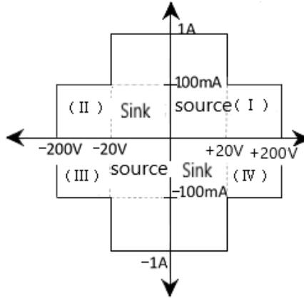
1A, 20V and 100mA, 200V amplitude is the nominal value. The actual maximum output voltage and output current amplitude are 1.05A, 21V and 105mA, 210V. The limit in the image above is not a range.
