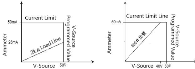
When the load resistor increases, the slope of the load line decreases. When the resistor increases to infinity (open circuit), the actual output voltage of the GSM is 50V and the output current is 0mA. When the load resistance decreases, the slope of the load line increases. When the resistance decreases to 0 (short circuit), the actual output voltage of the GSM is 0V and the output current is 50mA.
