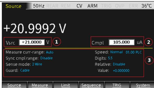
1. Source interface: the parameter setting consists of 3 areas, marked as ①②③ in the picture, press Edit/Lock key to toggle between ①②③.
