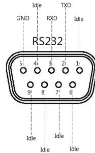
Parameters setting The RS-232 interface has 8 data bits, 1 stop bit, and no priority. The following RS232 communication parameters need to be set.
