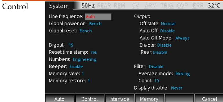
**Line frequency** Set the power line frequency according to the frequency of the power supply. It can be set as Auto, 50Hz or 60Hz. When setting to Auto, the GSM will detect the power line frequency and set it automatically when power on. When there is a lot of interference on the power line, you can manually set the frequency to avoid automatic detection of the wrong frequency that will affect the measurement result.
