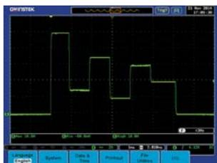
When operating the Sequence Function, PEL-3031E follows the time and load settings of step1, step2, step3, etc. so as to realize different load current variation.
