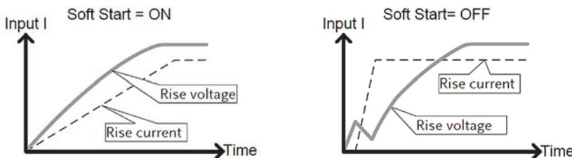
The soft start setting is used to limit the amount of input current at start-up. It can increase test reliability & stability.
