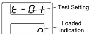
3. Rotate the Voltage knob to change the T setting (Test setting).
