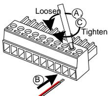
Unscrew the appropriate terminal anticlockwise to release the receptacle.
