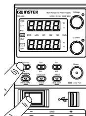
2. The display will show F-90 on the top and the configuration setting for F-90 on the bottom.
