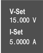
Parameter Settings Display Displays the parameter settings. For details on setting parameters, see page 20. The following figure shows the F1 parameter settings (V AND I), for example.
