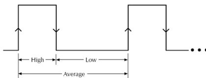
The high and average measurements are triggered by the rising edge of the pulse current and are performed for the time specified for the measurement.
