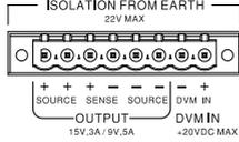
A total of 8 ports: 2 positive output terminals, 2 negative output terminals, a Sense+ terminal, a Sense- terminal, a DVM- input terminal and a DVM+ input terminal. Refer to the printed label under the terminals for the specific order of the terminals.
