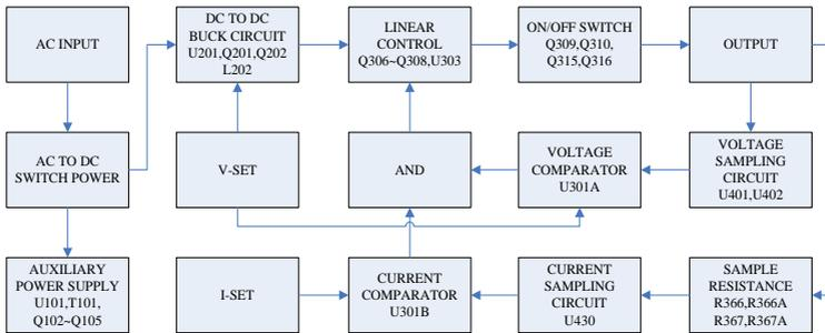
**Switching Power Supply**                      AC power is converted to 24VDC by the switch mode power supply module.
