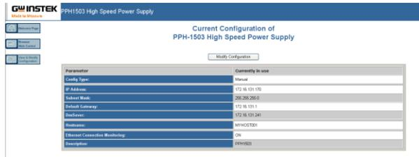
4. Click “Modify Config” to enter the network configuration setting menu, as shown below. Use the mouse to click on “Save and Restart” to change the remote settings for the PPH-1503.
