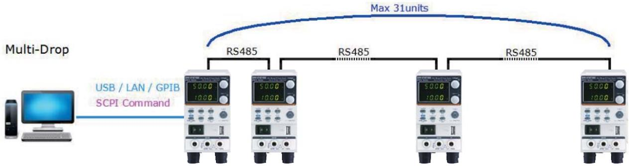
Provide USB, GPIB and LAN for PC to remote control Master PFR-100. RJ-45 connector on the rear panel can connect up to 31 units. LAN or USB remote control and augmenting slave
