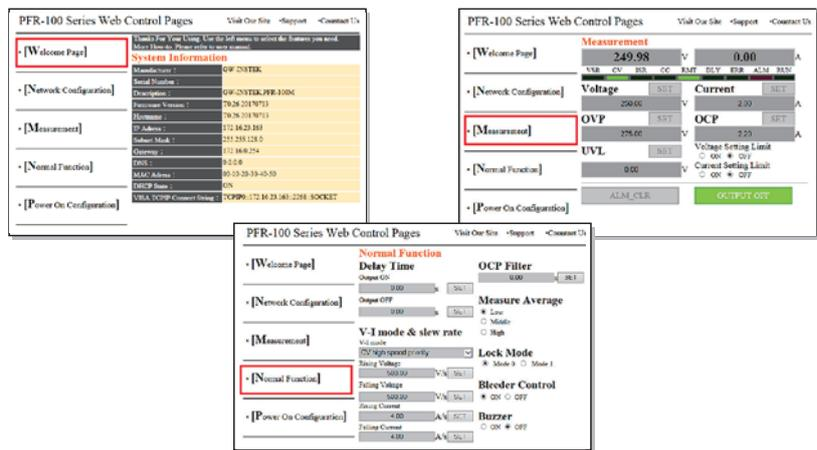
Users, via general browsers including Internet Explorer, Mozilla Firefox or Android cellular phones, can monitor PFR-100's test and measurement anywhere. Users not only can remotely monitor PFR-100 via internet, but also remotely observe and adjust your operating PFR-100 in the lab from your home. The outputs of PFR-100 can be monitored including OVP, OCP, UVL; and system
