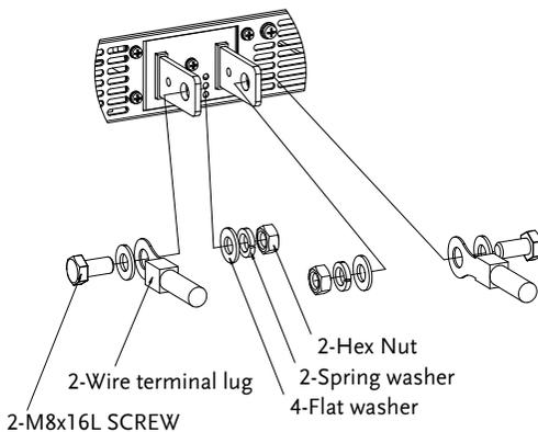
(PSU 100-15, 150-10, 300-5, 400-3.8, 600-2.6) Simply secure the stripped connectors inside each terminal.
