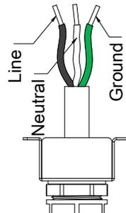
2. Make sure the sheath is tightened to the lock nut.
