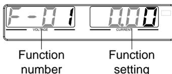
3. Rotate the Voltage knob to change the F setting to F-03 (V-I Mode Slew Rate Select).
