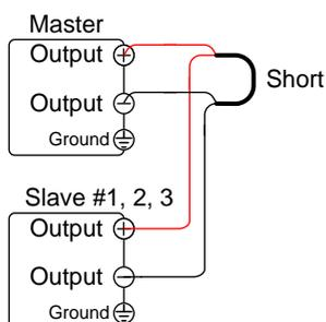
2. Connect the slave units to the master unit using the analog control connectors as described previously. Page 76
