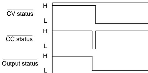
CV MODE: The diagram below shows the output status lines when the output is turned off in CV mode.
