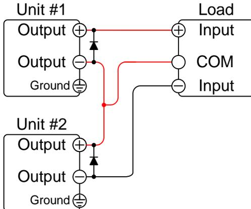
Note: The output reference ground (COMMON) can be grounded at the power supply side instead of the load, depending on the requirements. Local sensing should be used in this configuration.
