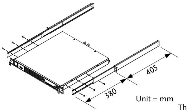
The following diagram shows the approximate dimensions of the GRM-001 sliding mounts. These sliding mounts should only be used within racks with a depth of 500mm.
