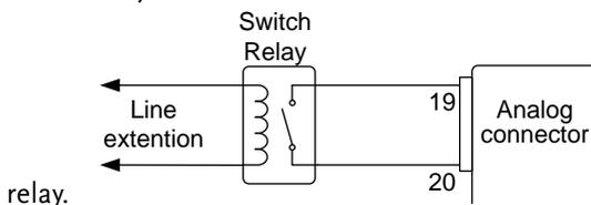
If a single switch control is to be used for multiple units, please isolate each instrument. This can be achieved by using a relay.
