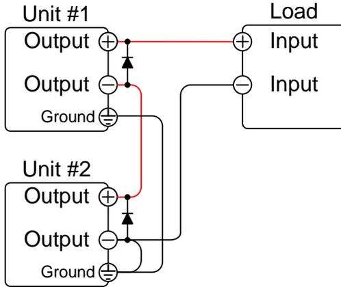
Series Connection to Output Positive and Negative Polarity
