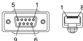
PSU-485 RS485 cable with DB9 connector
