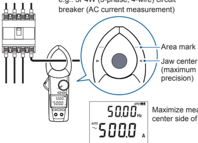
Maximize measurement precision by positioning the wire on the center side of the area mark.
