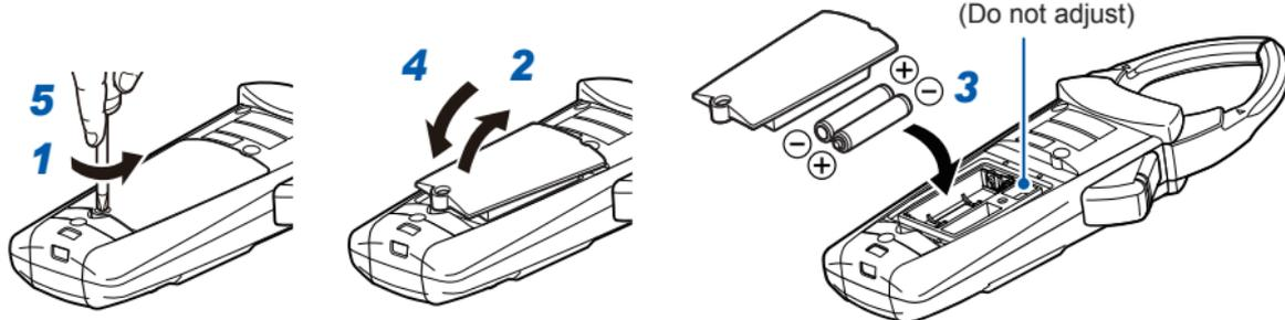
Do not adjust any screws other than the screw holding the battery cover in place. Do not adjust the three screws underneath the cover, which are used to adjust measured values, as doing so may prevent accurate measurement.
