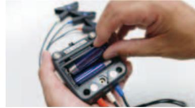
Two AA batteries deliver 70 hours of continuous use. This long service life means fewer troublesome battery changes. In addition, there's no need to carry spare batteries.
