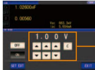
The generated voltage can be varied from 0 V to 2.50 V DC (10 mV resolution).
