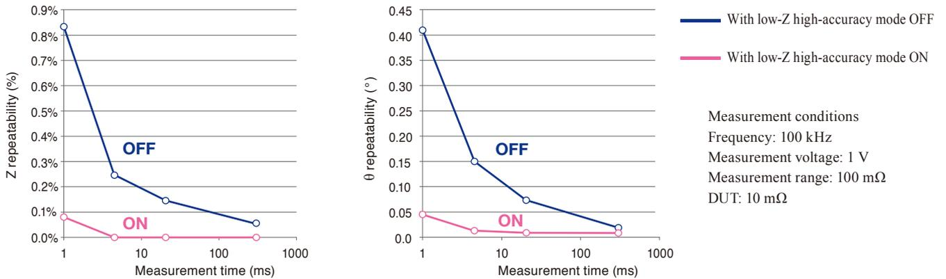
Low-Z high-accuracy mode can be used with the 100 mΩ, 1 Ω, and 10 Ω ranges.
