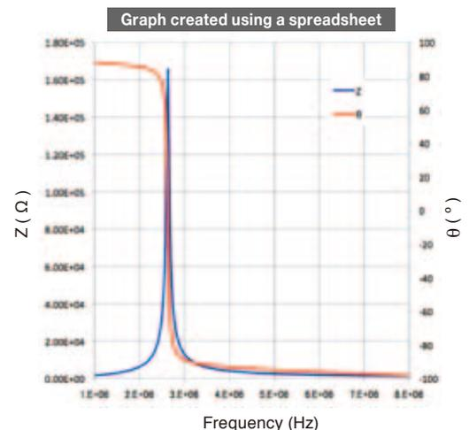
The IM3536 ships standard with application software that can save measurement data as an Excel file while sweeping through a range of frequencies pre-configured on a computer.
