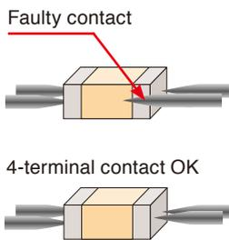
The contact check function measures the contact resistance between L<sub>POT</sub> and L<sub>CUR</sub> and between H<sub>POT</sub> and H<sub>CUR</sub> and displays an error if the readings are greater than or equal to a preset threshold.
