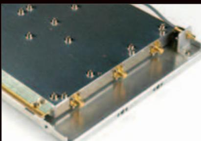
Each section uses a solid shield carved to match the on-board pattern or IC shape, thus reducing internal coupling. The shield also reduces external radiation and improves noise resistance, meeting a high level of EMC, despite being the lightest in its class.
