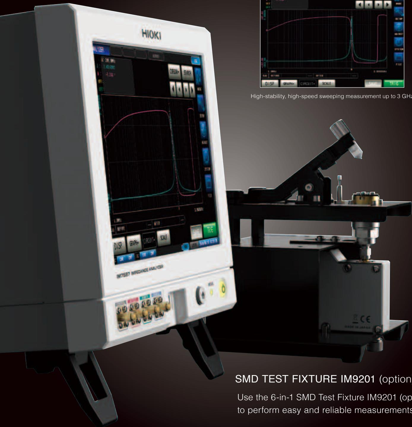
High-stability, high-speed sweeping measurement up to 3 GHz
