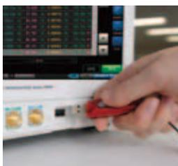
Save measurement conditions and results in a USB flash drive
