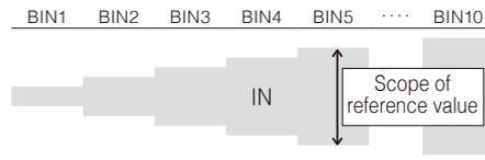
Set upper and lower limits for each bin. The impedance analyzer will rank components using up to 10 categories. \*Upper and lower limit settings are the same as for comparator measurement.
