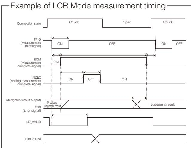
\*In this example, the TRIG signal's active edge is the falling edge (ON).
