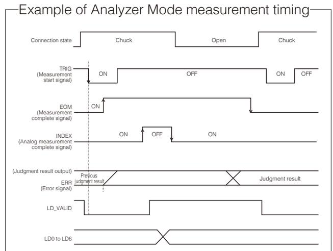
EOM: Off from trigger input to end of measurement processing
