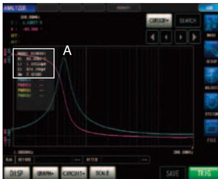
Analyze individual component values (L/C/R) for elements in the following five circuits based on measurement results.
