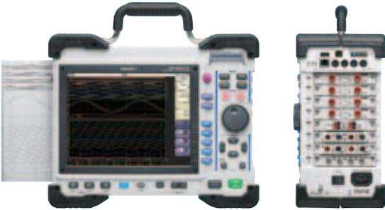
Note: Main unit MR8847A cannot operate alone. You must install one or more optional input modules in the unit.
