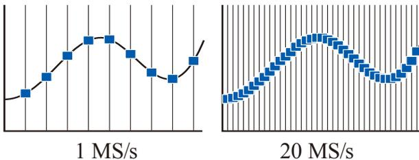
High-speed sampling allows you to measure the rising edge of pulses and detect anomaly operations and instantaneous waveforms that occur suddenly with high precision.
