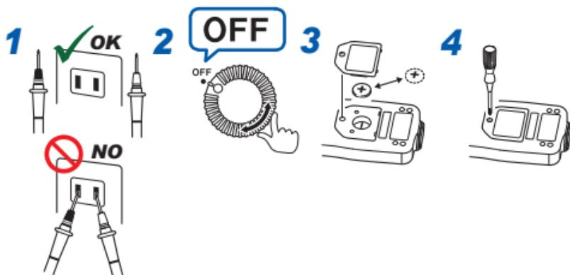
Do not turn the adjustment screw inside the battery case. Doing so will cause the instrument to report abnormal measured values.
