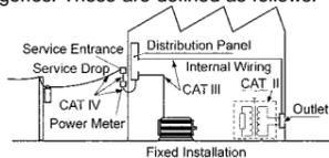
Using a measurement instrument in an environment designated with a higher-numbered category than that for which the instrument is rated could result in a severe accident, and must be carefully avoided.
