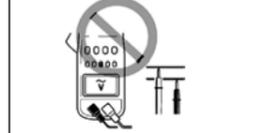
Avoid touching the exposed metallic parts of the clamp sensor while measuring voltage.
