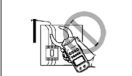
Do not input voltage in the resistance measurement, continuity checking and temperature measurement.
