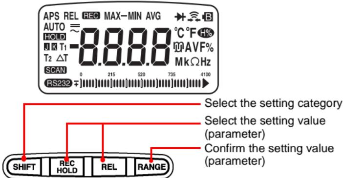
1. In order to display the setting screen hold down the **SHIFT** key and turn the unit on by turning the function switch from the OFF position.
