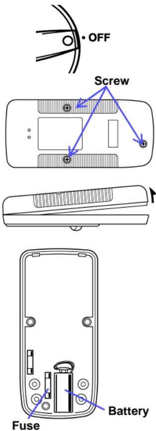
1. Disconnect the test leads from the unit and set the function switch to OFF.
