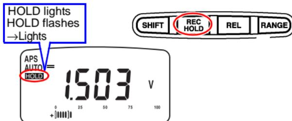
To cancel the trigger hold function, press and hold the **REC/HOLD** key.
