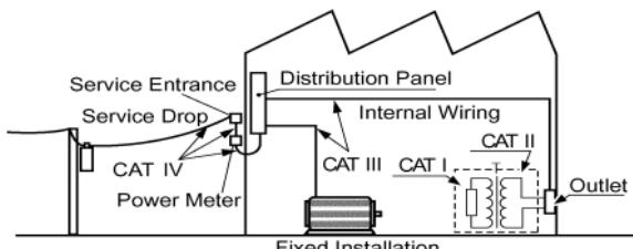
Higher-numbered categories correspond to electrical environments with greater momentary energy. So a measurement device designed for CAT III environments can endure greater momentary energy than a device designed for CAT II.
