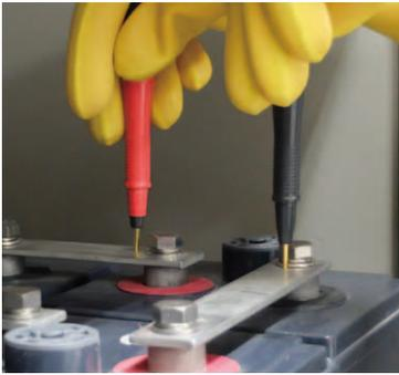
When the measured value stabilizes, save it automatically without having to operate the switch. Wait time can be as short as only 2 seconds to auto-save from when the test leads make contact with the battery terminals, **cutting time by 60%** compared to the legacy product.
