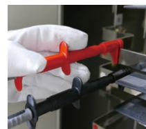
For clamping around the target busbar
