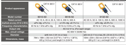
Adapter Model 9704 is required to connect AC CLAMP ON PROBES 9010-50, 9018-50 and 9132-50 to the DT4281, DT4261, DT4253, DT4255, DT4256.
