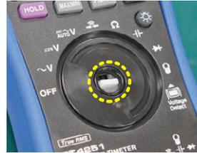
If dust gets into the instrument's enclosure, it can cause the device to fail. Since dust can get into the instrument especially easily through the gap around the rotary switch, the DT4200 series incorporates a dust-proof part known as an O-ring where the rotary switch is mounted to improve the device's dust resistance.
