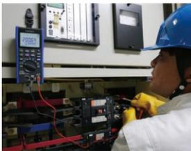
The DT4200 series features a display with a wide viewing angle and a backlight function so that it's easy to read, even when you can't view the screen from the front or when making measurements in a dim location.
