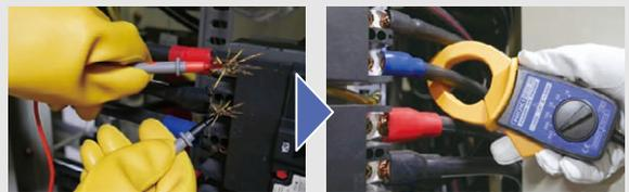
The DT4281, DT4261, DT4253, DT4255 and DT4256 eliminate the root cause of such accidents by providing clamp-on sensor-based current measurement functionality instead of using conventional probes.
