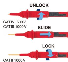
Test leads L9300 now incorporate integrated caps. The design lets you change the measurement category simply by sliding the test lead's protective finger guard. As an added bonus, you no longer have to worry about losing caps!
