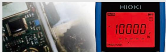
To prevent an accident, a warning function immediately notifies the operator if the DMM receives excessively high input.
