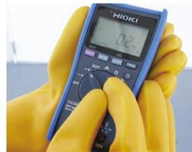
The DT4200's rotary switch is designed to be easy to turn even when wearing thick work gloves, for example while working in hazardous measurement locations or harsh conditions.
