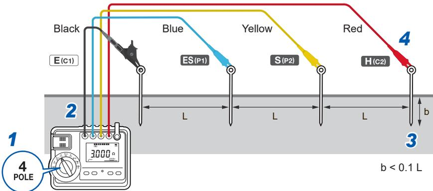
Always execute a zero adjustment before measurements. (p.82)
