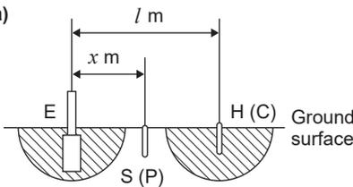
Resistance area of the earth resistance under measurement ( $R_x$ )
