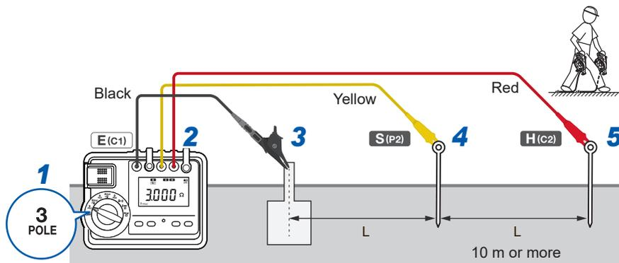
Disconnecting the earth electrode from the installation allows the instrument to measure earth-resistance values correctly. Disconnect the earth electrode from the installation before starting a measurement. If the earth electrode cannot be separated from the equipment, make measurements using the three-pole MEC measurement.
