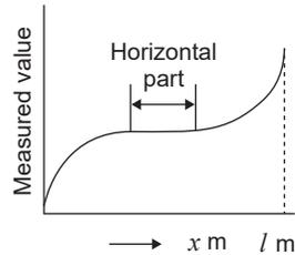
Electrodes E and H (C) can be separated up to 50 m by using the optional L9843-51, L9843-52, or L9843-53. Electrode S (P) can also be separated from Electrode E within the distance where the horizontal part is found shown in Fig. (b). Measurements can be made, in principle, even if they are separated more than 50 m; however, the measurement results cannot be guaranteed.
