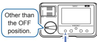
Turn on the instrument while holding down
