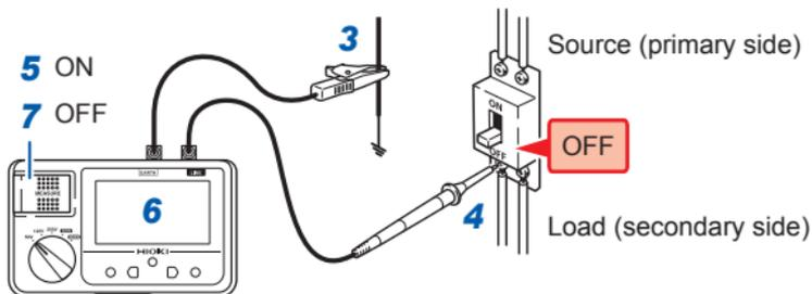
**3** Connect the black test lead to the ground side of the object being measured.
