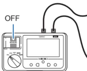
Without removing the test leads from the measurement object, turn off the **MEASURE** key.
