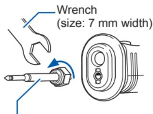
**2 Remove the tip pin by rotating with a wrench.**
