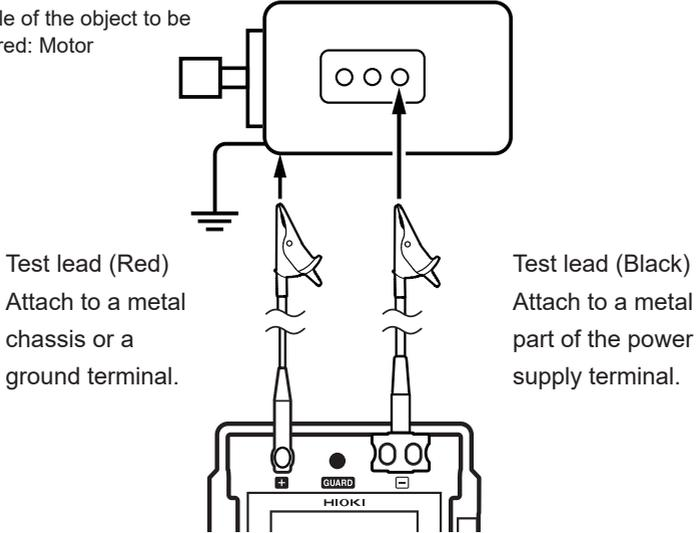
**4** Hold down the **MEASURE** key for more than one second to start measurement.
