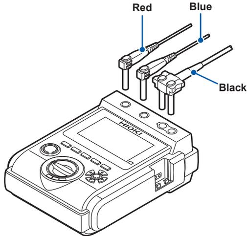
\*1. A **GUARD** terminal is used to prevent the surface electrical resistance of an insulating material affecting measurement, enabling correct measurement of the entire volume resistivity of the material. See “3.6 Use of GUARD Terminal” (p. 48).
