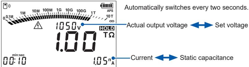
When measuring for 1 min. or more, the 1-min. value can be displayed with the ◀ or ▶ key, either during or after measurement.
