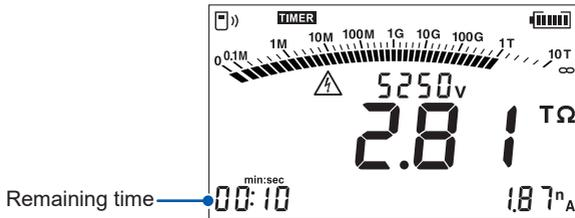
After the set time has elapsed, the instrument automatically stops measurement.
