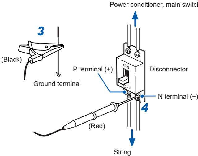
There is a risk of insulation deterioration when voltage is generated between the N terminal and ground. When there is voltage in the object under measurement, the backlight blinks in red by the voltage detection function.
