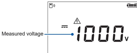
You can retain the measured value by pressing the **MEASURE** key. (**[HOLD]** lights up.)
