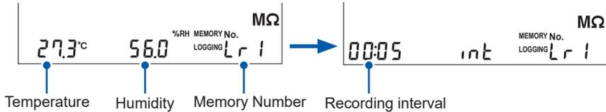
The instrument is in the measurement standby state.
