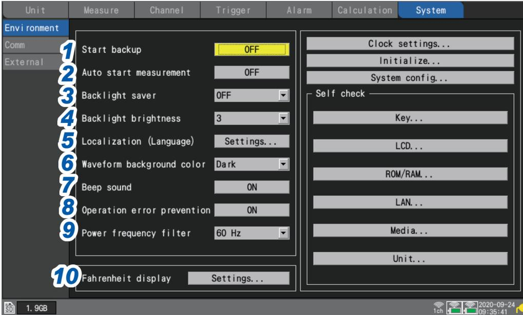
**1 Under [Start backup], select the operation to perform when the instrument is turned back on (start back up).**
