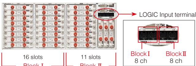
Block I : Analog 32ch, Logic 8ch
