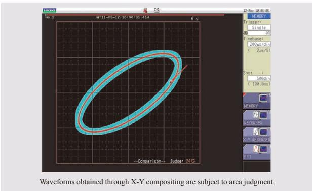
The MR8741 includes functionality for judging X-Y waveforms. Waveforms measured using the memory function and created with X-Y compositing are subject to area judgment.
