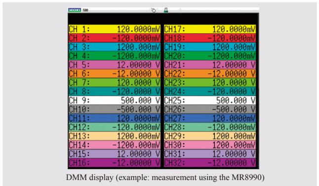
Input values can be monitored numerically in the manner of a digital multimeter (DMM).
