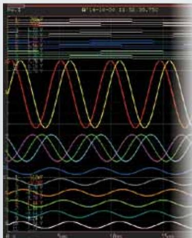
Conventional devices used a 640x480 dot TFT LCD, but the next-generation MR8827 uses an 800x600 dot SVGA high resolution LCD to make it even easier to identify overlapping measured waveforms.
