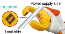
**FAIL** The I vector's phase direction is opposite the determination area.
