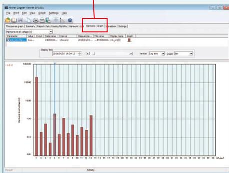
Configure the PW3365's settings to save waveforms and display them using the SF1001.
