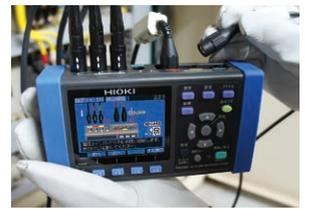
**STEP3** Connect the voltage sensor
