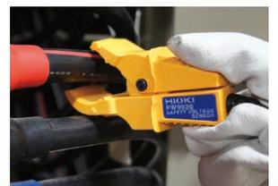
**STEP4** Connect the clamp sensors
