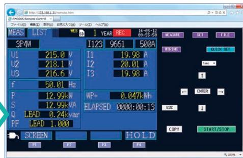
Display the power logger's screen and make adjustments virtually by clicking the buttons and entering new information.
