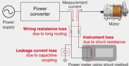
The wiring of the measurement target is routed for connecting to the current input terminal. However, this results in an increase in the influence of power loss from wiring resistance and capacitive coupling, and meter loss ing due to shunt resistance. All of this loss leads to larger degradation in accuracy.
