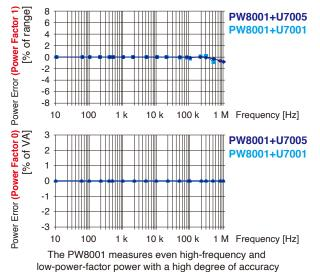
Accurate capture of power fluctuations caused by high-speed switching
