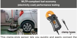
instrument for measurement. It's used in testing of assembled vehicles where it would be difficult to cut wires. Capable of withstanding temperatures of -40°C to 85°C, the device can be used in the hot environment of an engine compartment.
