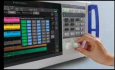
Adjust the displayed waveform position, triggers, and harmonic orders with intuitive knob-based operation.
