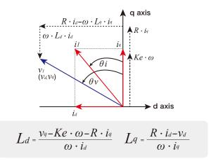
*Ld* and *Lq* impedance values in the *d*- and *q*-axis directions are calculated based on the results of analyzing the *d*-axis and *q*-axis voltage and current vectors.
