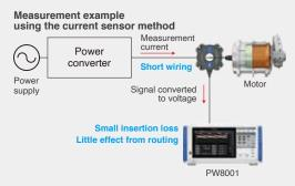
A current sensor is connected to the wiring on the measurement target. This reduces the effects of wiring and loss on the side of the measurement instrument. This allows measurements with wiring conditions that are close to the actual operating environment of a highly efficient system.
