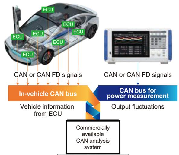
**6 Observation of analog signals, CAN signals, and power fluctuations on the same time series**
