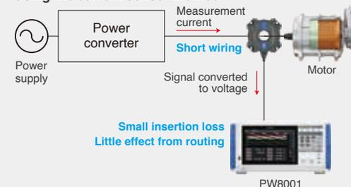
A current sensor is connected to the wiring on the measurement target. This reduces the effects of wiring and loss on the side of the measurement instrument. This allows measurements with wiring conditions that are close to the actual operating environment of a highly efficient system.
