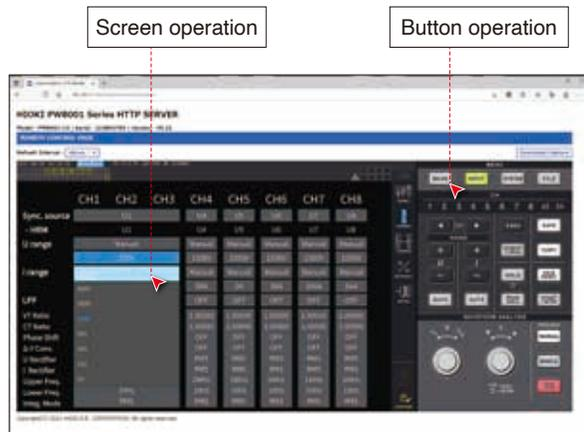
When a PW8001 is connected simultaneously to four PCs, only one of them can control the instrument.
