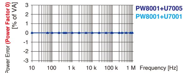
The PW8001 measures even high-frequency and low-power-factor power with a high degree of accuracy
