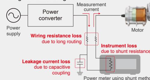
The wiring of the measurement target is routed for connecting to the current input terminal. However, this results in an increase in the influence of power loss from wiring resistance and capacitive coupling, and meter loss due to shunt resistance. All of this loss leads to larger degradation in accuracy.
