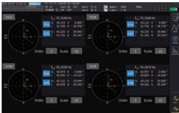
**Example of 4-inverter-motor analysis with a 3P3W2M connection**
