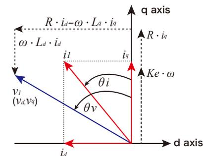
$$L_d = \frac{v_q - Ke \cdot \omega - R \cdot i_q}{\omega \cdot i_d} \quad L_q = \frac{R \cdot i_d - v_d}{\omega \cdot i_q}$$
