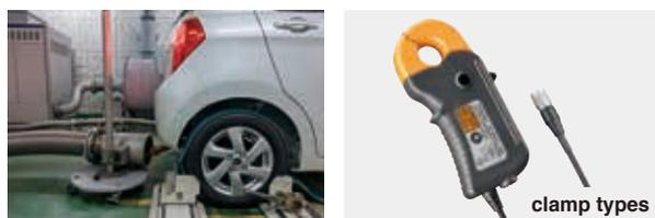
This clamp-style sensor lets you quickly and easily connect the instrument for measurement. It's used in testing of assembled vehicles where it would be difficult to cut wires. Capable of withstanding temperatures of -40°C to 85°C, the device can be used in the hot environment of an engine compartment.
