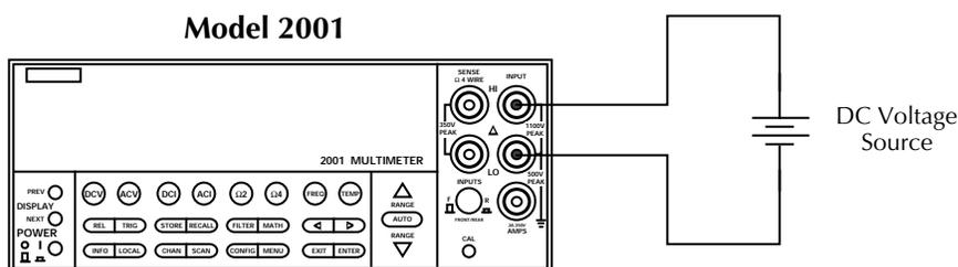
Input Resistance = 10M $\Omega$  on 1000V and 200V ranges ;
