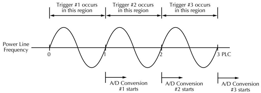
Note: A/D conversions assume an integration time of  $\leq 1$  PLC (Power Line Cycle)
