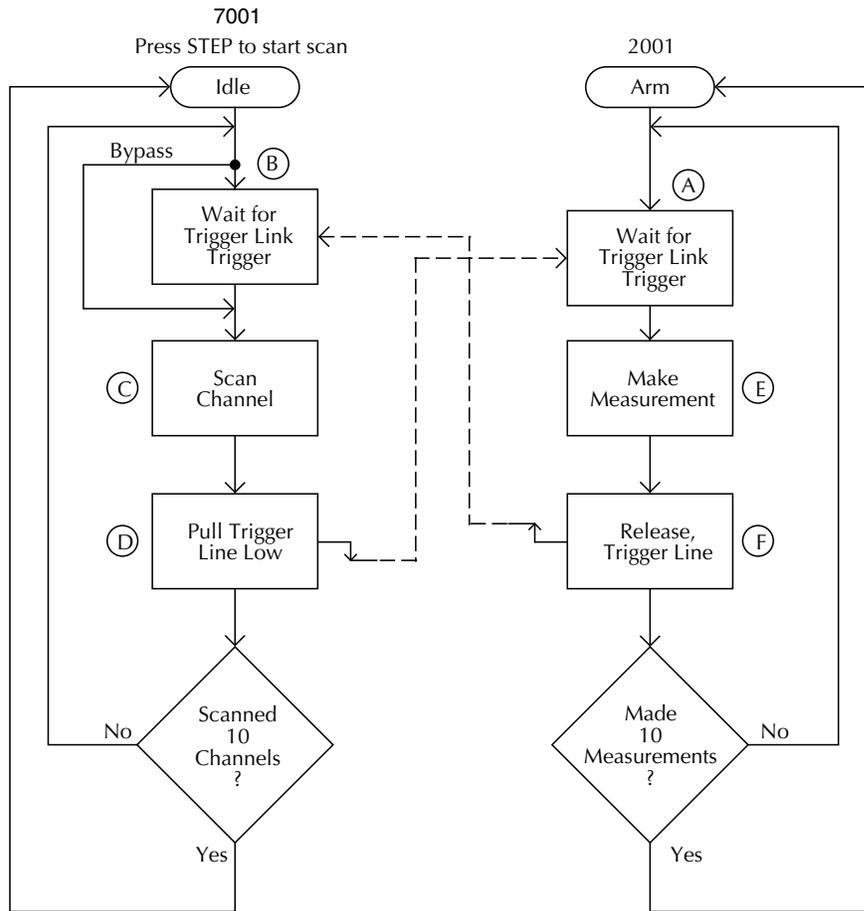
Figure 3-39 Operation mode for semi-synchronous Trigger Link example
