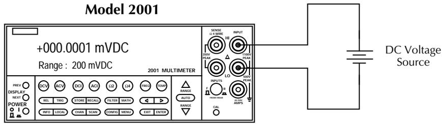
Input Resistance = 10MΩ on 1000V and 200V ranges ;
