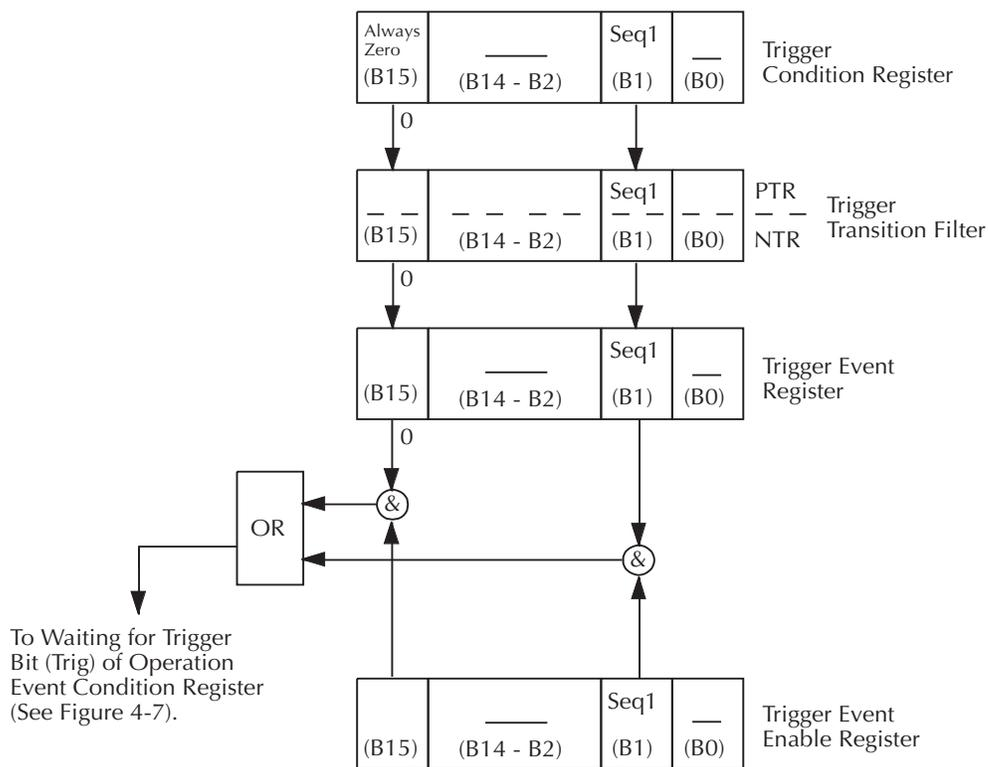
Seq 1 = Sequence 1 (Set bit indicates that the 2001 is in the trigger layer of Sequence 1)
