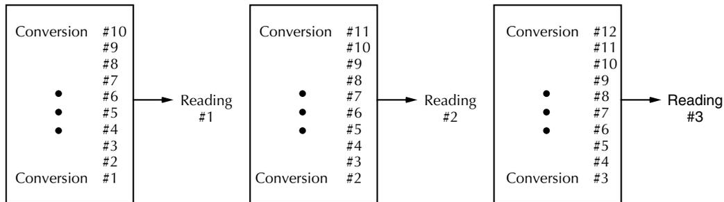
**B. Moving filter mode; Type - Average, Readings = 10**
