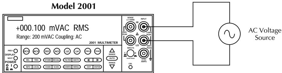
Input Impedance = 1MΩ shunted by <140pF
