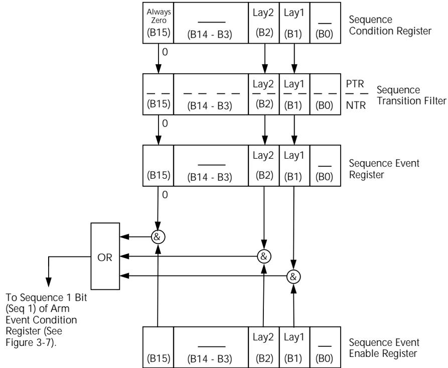
Lay1 = Layer 1 (Set bit indicates that 2002 is in arm layer 1).
