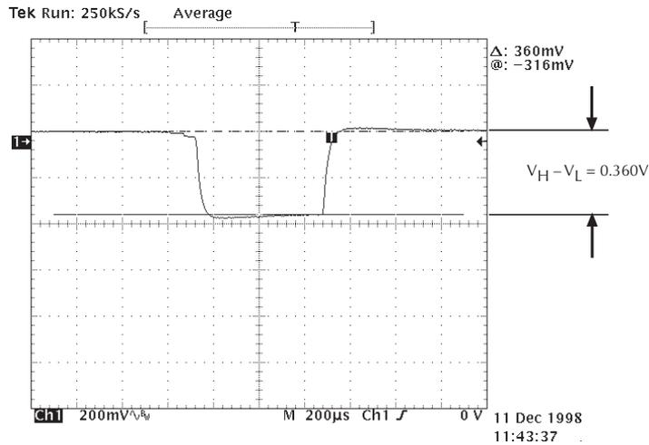
NOTE Figure E-7 contains the voltage drop during the transmit portion of the pulse of a GSM phone with the Model 2306 battery channel, output impedance set to  $0.24\Omega$ .
