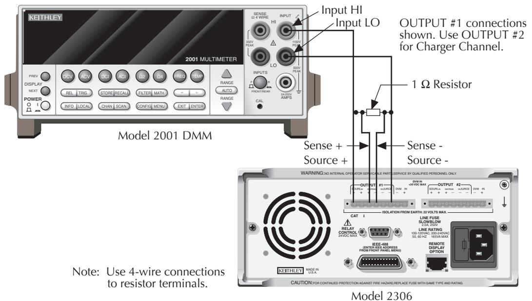
2. Select the multimeter DC voltage measuring function, and enable auto-ranging.
