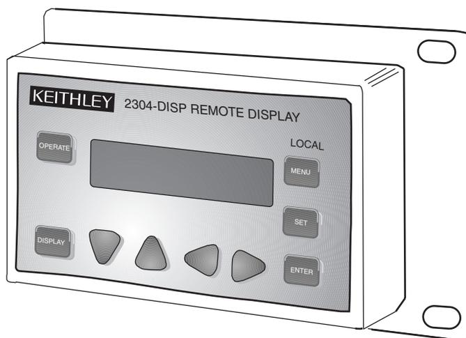
*NOTE* When using the remote display, VFD BRIGHTNESS may not appear in the main menu (dependent on the firmware revision in the unit).
