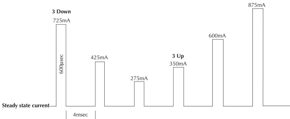
For the active steps, the trigger level may be set to a value appropriate for each rising or falling step, or set to the same value for all active steps. If using the same values for all TLEV<sub>x</sub> steps, make sure the TLEV value set is appropriate for the smallest step (in [Figure 3-8](#), the TLEV value could not be greater than 275mA). See [Table 3-5](#) for sample trigger level values.
