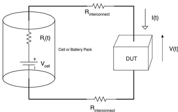
If  $R_{\text{interconnect}}$  is small compared to  $R_i(t)$  and  $R_i(t)$  is relatively constant during the length of the pulse,  $R_i(t) \sim R_i$ , then the voltage across the DUT may be expressed as:
