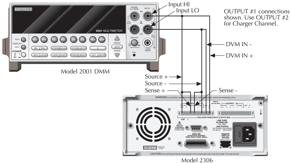
1. Select the DMM DC volts function, and enable auto-ranging.
