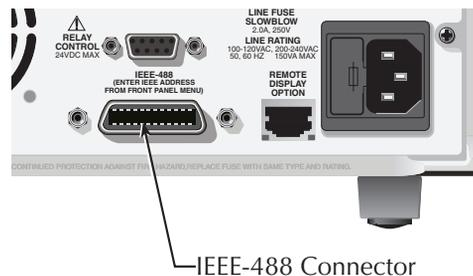
**NOTE** To minimize interference caused by electromagnetic radiation, use only shielded IEEE-488 cables. Available shielded cables from Keithley are Models 7007-1 and 7007-2.
