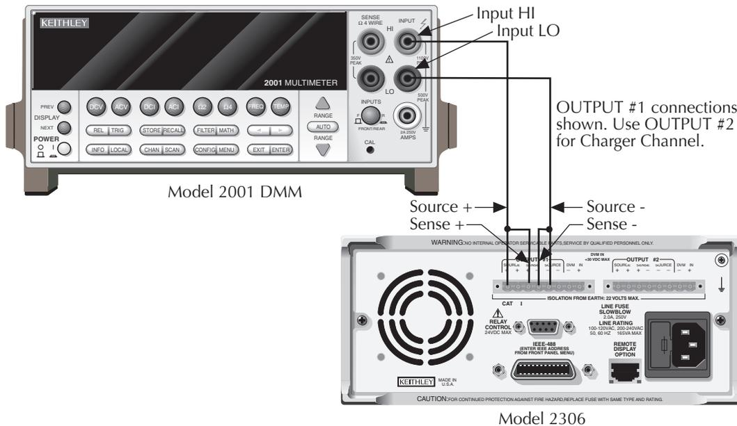
2. Select the multimeter DC volts measuring function, and enable auto-ranging.
