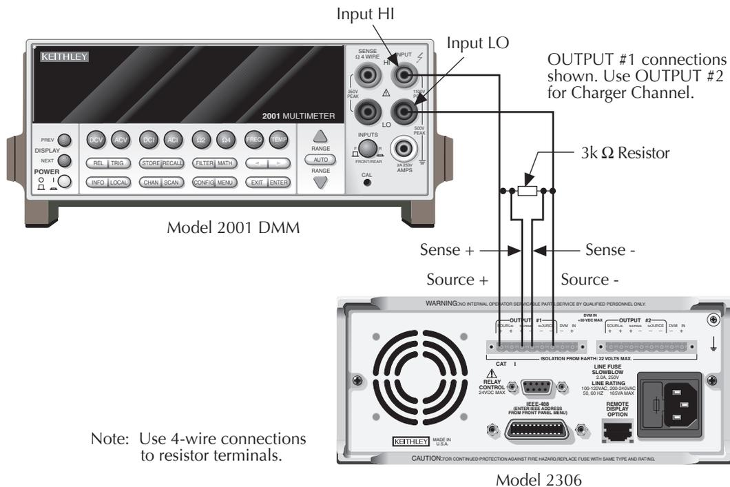
2. Select the multimeter DC volts measuring function, and enable auto-range.
