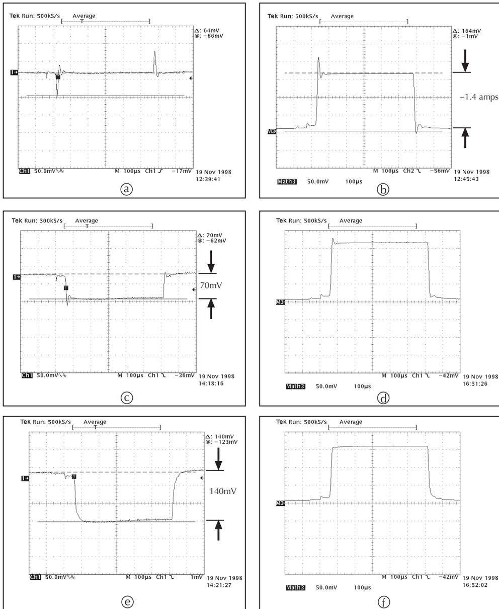
**NOTE** *Figure E-5 contains the effect of the variable output impedance control of the Model 2306 on the current and voltage performance of a GSM handset.*
