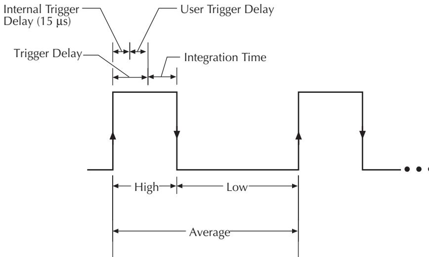
*High* = integration time specified for high measurement time + *Trigger Delay*
