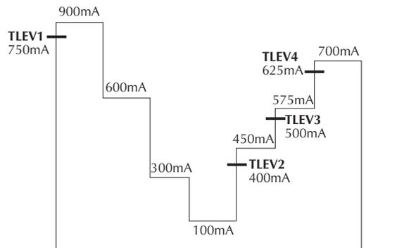
To measure the up step values in this pulse sequence, set the value for UP steps to equal the sum of actual UP steps plus one while setting the DOWN step value to zero. In [Figure 3-9](#), the UP steps are set to 4 and DOWN steps to 0. (If UP steps are set to a non-zero value, the
