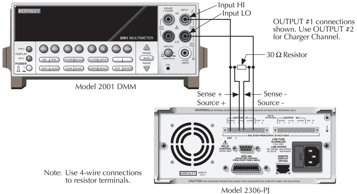
2. Select the multimeter DC volts measuring function, and enable auto-range.
