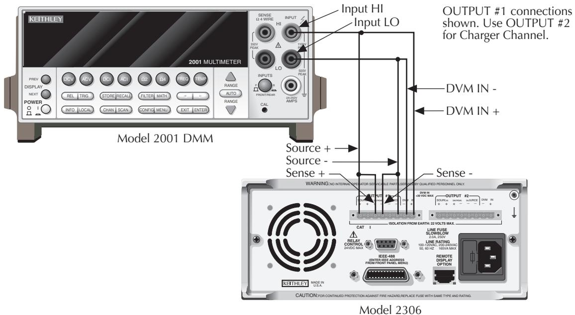
3. The unit will prompt you for the DMM reading, which will be used to calibrate the Channel #1 full-scale output voltage:
