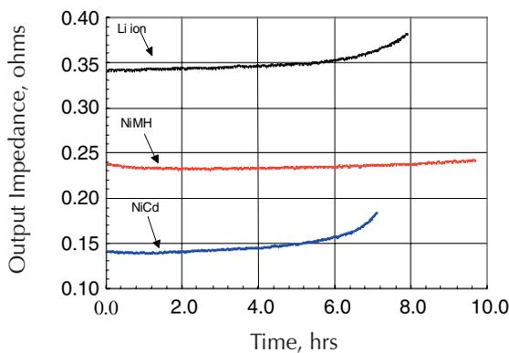
**NOTE** Figure E-4 shows electronic resistance for battery packs during a simulated GSM phone pulsed discharge from full charge to 5.5 volts.
