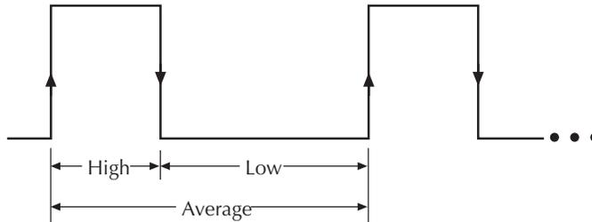
↑ High and average measurements triggered on leading edge of pulse
