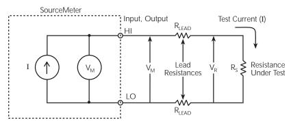
I = Current sourced by SourceMeter  $V_M$  = Voltage measured by SourceMeter  $V_R$  = Voltage across resistor Measured resistance =  $\frac{V_M}{I}$  =  $R_S$  + (2 ×  $R_{LEAD}$ ) Actual resistance =  $\frac{V_R}{r}$  =  $R_S$
