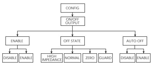
Figure 13-5 **Output configuration menu tree**
