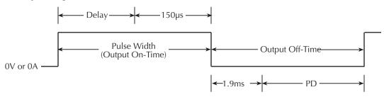
Delay = Pulse width delay, used to achieve pulse width setting.
