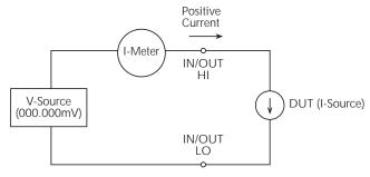
Note: Positive current flowing out of IN/OUT HI results in positive (+) measurements.
