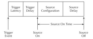
Trigger Latency: 225µsec max Source Configuration: 50µsec max
