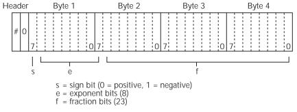
Normal byte order shown. For swapped byte order, bytes sent in reverse order: Header, Byte 4, Byte 3, Byte 2, Byte 1.
