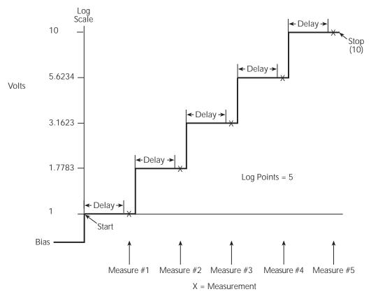
The programmable parameters for a log sweep include the start and stop levels and the number of measurement points for the sweep. The specified start, stop, and point parameters determine the logarithmic step size for the sweep. Step size for the sweep in Figure 10-2 is calculated as follows:
