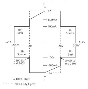
Figure 6-4 Model 2410 operating boundaries (T<sub>amb</sub> №C)
