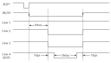
\* With the SOT line being pulsed low (as shown), ↓ STEST must be the selected event for the trigger model. If the SOT line is instead pulsed high by the handler, ↑ STEST must be the selected arm event. For high or low pulses, select ↑↓STEST.
