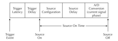
Trigger Latency: 225µsec max Source Configuration: 50µsec max
