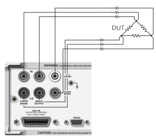
C. 6-wire ohms connections
