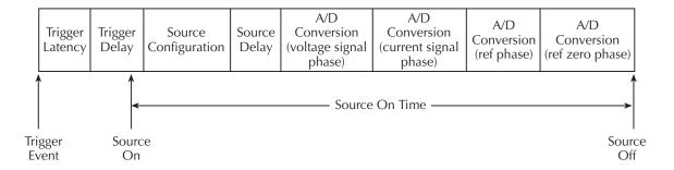
Trigger Latency: 225µsec max Source Configuration: 50µsec max
