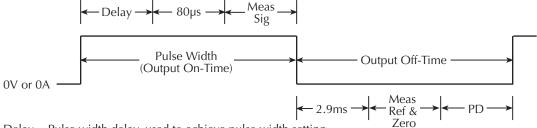
Delay = Pulse width delay, used to achieve pulse width setting. 80µs = Minimum pulse width overhead
