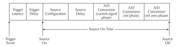
Trigger Latency: 225µsec max Source Configuration: 50µsec max
