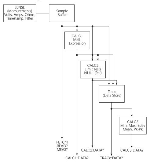
The SENSE block represents the basic measured readings of voltage, current, and resistance. If Filter is enabled, the readings will be filtered. The SENSE block also measures time for the timestamp.
