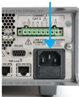
3. Connect the plug of the power cord to a grounded AC outlet.
