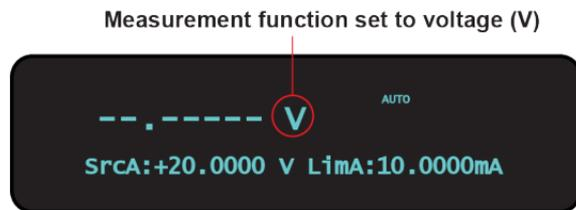
2. Press the AUTO
