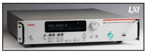
The high power Model 2651A is the newest addition to the Series 2600A family of System SourceMeter instruments. Specifically designed to characterize and test high power electronics, these source measurement unit (SMU) instruments can help you improve productivity in applications across the R&D, reliability, and production spectrums, including high brightness LEDs, power semiconductors, DC-DC converters, batteries, and other high power materials, components, modules, and subassemblies.
