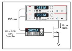
Keithley's TSP and TSP-Link technology enables true SMU-per-pin testing without the power and/or channel limitations of a mainframe-based system.
