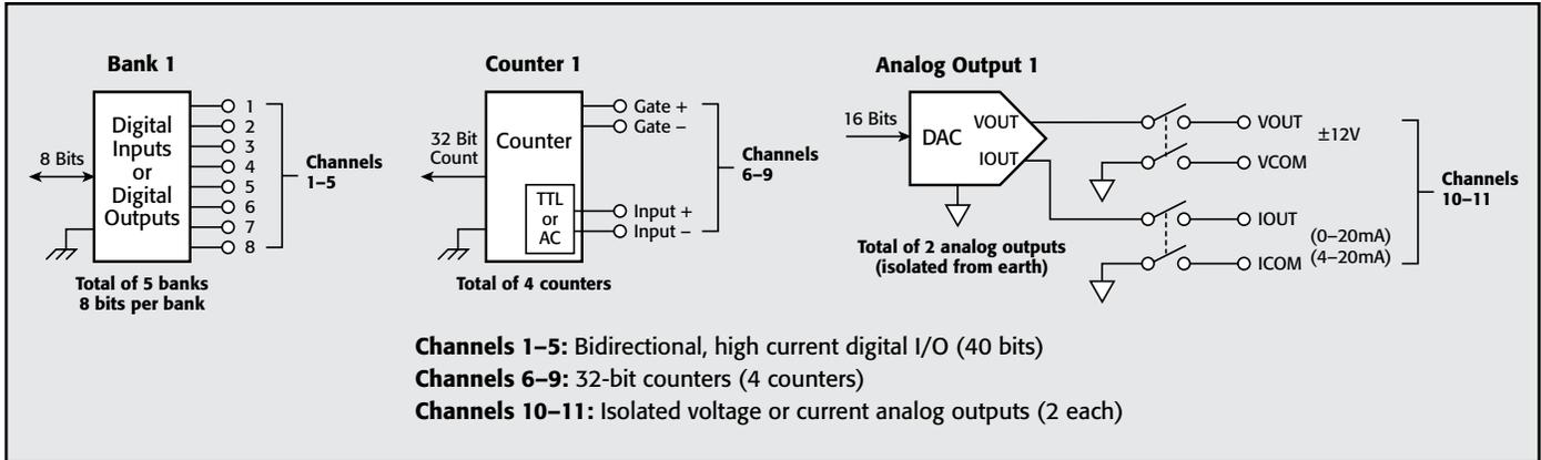
Figure 1. Block diagram
