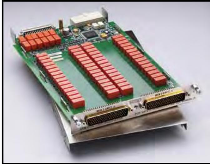
The Model 3720 offers two independent banks of 1×30 two-pole multiplexers. It is ideal for general purpose switching, including temperature measurements. The two banks can automatically be connected to the Series 3700 mainframe backplane and optional DMM through the analog backplane connection relays. This connection allows the mainframe to reconfigure the card to a single 1×60 two-pole multiplexer or to enable card-to-card expansion for even larger configurations.
