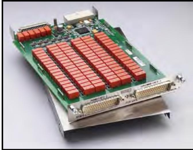
The Model 3730 is a two-pole, 6 row by 16 column matrix card. It can connect up to six differential instrument channels to any combination of 16 DUTs (devices under test). Any row can be connected to the Series 3700 mainframe backplane by using the analog backplane connection relays. This allows for easy matrix column expansion. A matrix of up to 6 rows by 96 columns can be supported within a single Model 3706 mainframe (with six Model 3730 cards).
