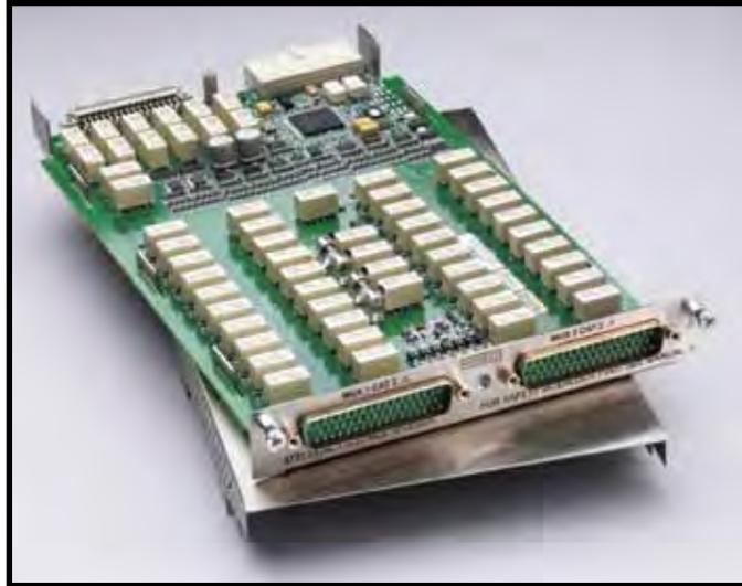
The Model 3721 offers two independent banks of 1x20 two-pole multiplexers that are ideal for general purpose switching, including temperature measurements. The two banks can automatically be connected to the Series 3700 mainframe backplane and optional DMM through the analog backplane connection relays. This connection allows the mainframe to reconfigure the Model 3721 as a single 1x40 two-pole multiplexer or to enable card-to-card expansion for even larger configurations.
