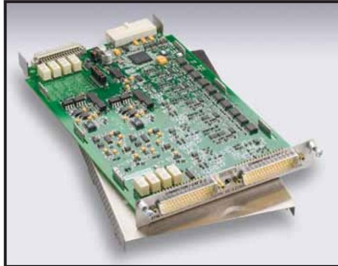
Use the Model 3750 to monitor and control your automated test system. The flexibility and speed provided by the 40 digital I/O bits, four counters, and two analog outputs make it well-suited for a wide variety of system control applications.
