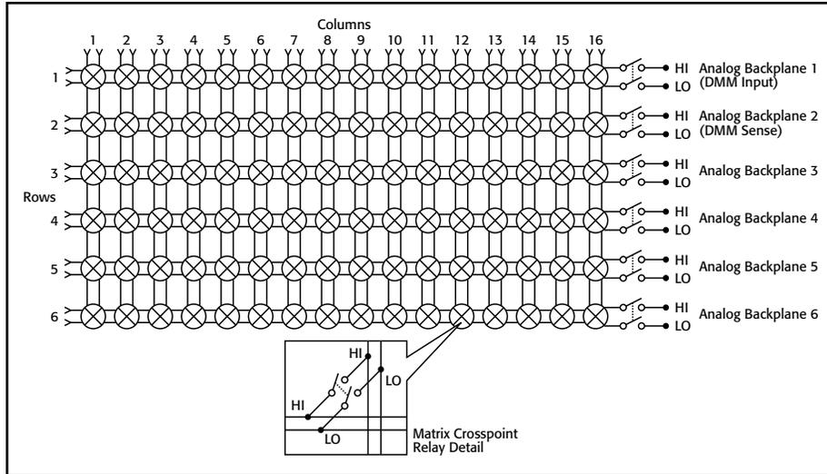
**MATRIX CONFIGURATION:** 6 row by 16 column matrix. Columns can be expanded using the backplane or isolated by relays.
