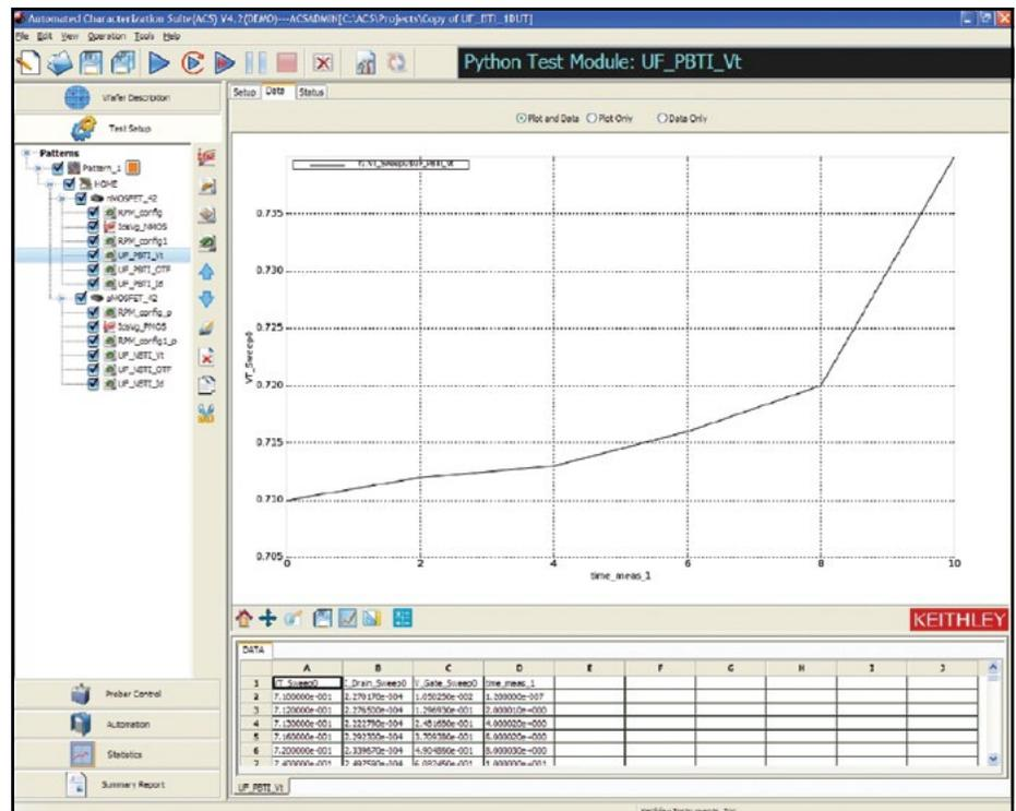
The Model 4225-PMU/4225-RPM's combination of superior speed and sensitivity allow characterizing voltage threshold ( $V_T$ ) directly with high-speed  $I_D$ - $V_C$  sweeps. Measuring  $V_T$  directly makes it unnecessary to correlate the single-point  $I_D$  measurement to actual  $V_T$  levels.
