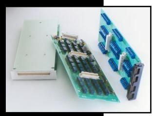
the 7011 to switch 4-pole signals by combining channel pairs. This gives you a dual 1×10 4-pole multiplexer or a single 1×20 4-pole multiplexer. Each of the four multiplexer outputs on this card connects to the 7001/7002 analog backplane through removable jumpers for even greater flexibility. Two 7011 cards can be used to make a single 1×80 multiplexer with all intercard connections through the backplane. The 7011 multiplexer outputs can also be
