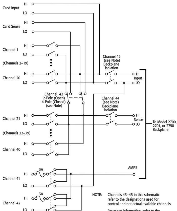
**NOTE:** Channels 43–45 in this schematic refer to the designations used for control and not actual available channels. For more information, refer to the ROUTe:MuLTiple command section in the Model 2700, 2701, or 2750 User's Manual. Channels 44 and 45 can be individually controlled using ROUTe:MuLTiple if the module is not to be connected to the internal DMM.
