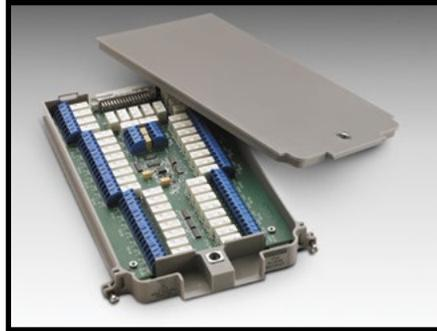
The Model 7702 plug-in module offers 40 channels of 2-pole or 20 channels of 4-pole multiplexer switching that can be configured as two independent banks of multiplexers. The Model 7702 provides two additional protected channels for current measurements. It is ideal for RTD, thermistor, and thermocouple temperature applications.
