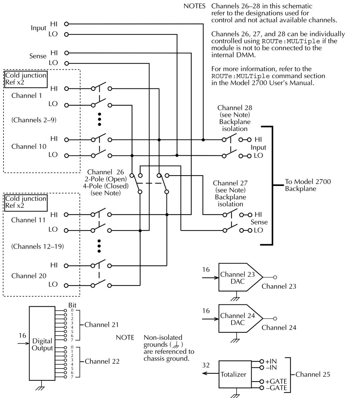
NOTES Channels 26-28 in this schematic refer to the designations used for control and not actual available channels.
