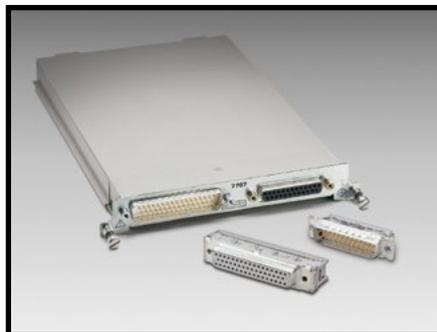
The Model 7707 plug-in module offers 10 channels of 2-pole or 5 channels of 4-pole multiplexer switching that can be configured as two independent banks of multiplexers. The Model 7707 also provides 32 digital input/output channels (four 8-bit ports) for I/O control. Connect the Model 7707 to industry standard solid-state relays to switch up to 980VA.
