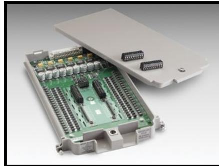
The Model 7710 plug-in module offers 20 channels of 2-pole or 10 channels of 4-pole relay input that can be configured as two independent banks of multiplexers. The relays are solid state, providing long life and low maintenance. Solid-state relays usually have 100 times longer life than mechanical relays. It is ideal for long-term data logging applications as well as for demanding high-speed applications.
