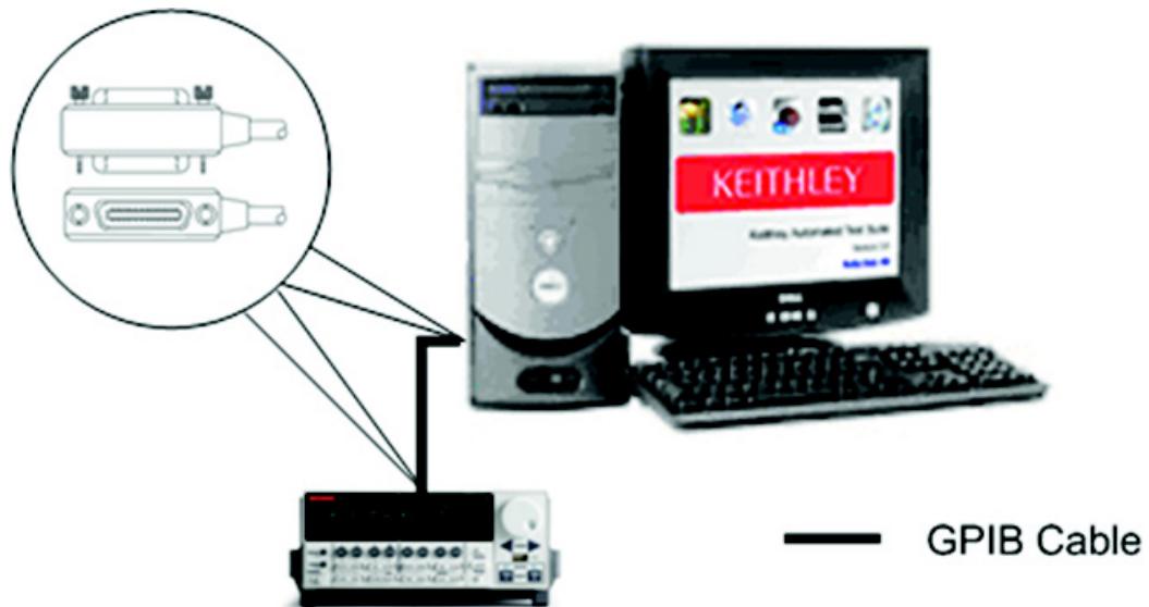
Figure 24: Single instrument GPIB configuration
