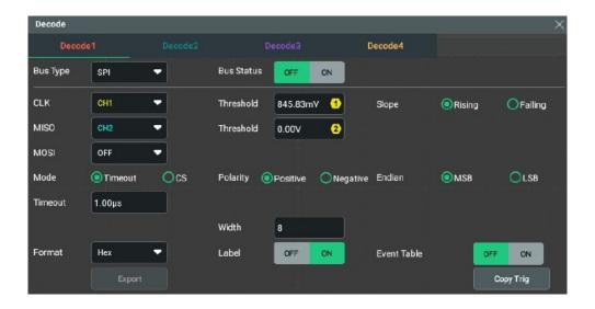
Figure 15.11 SPI Decoding Menu
