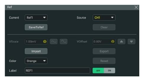
Figure 13.1 Reference Waveform Menu
