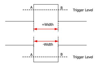
Figure 8.4 Positive/Negative Pulse Width
