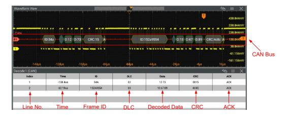
Figure 15.15 CAN Decoding Event Table
