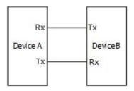
Figure 15.4 Schematic Diagram of RS232 Serial Bus
