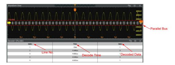
**Figure 15.3 Parallel Decoding Event Table**
