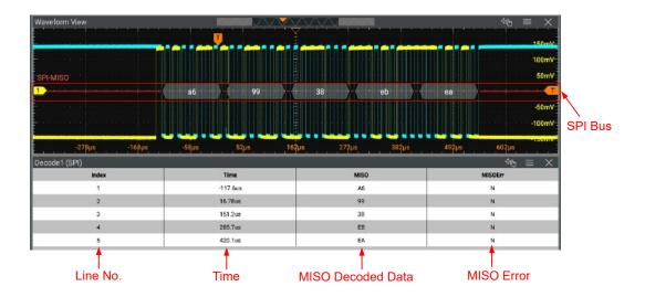
Figure 15.12 SPI Decoding Event Table
