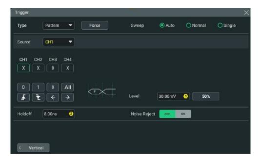
Figure 8.10 Pattern Trigger Setting Menu
