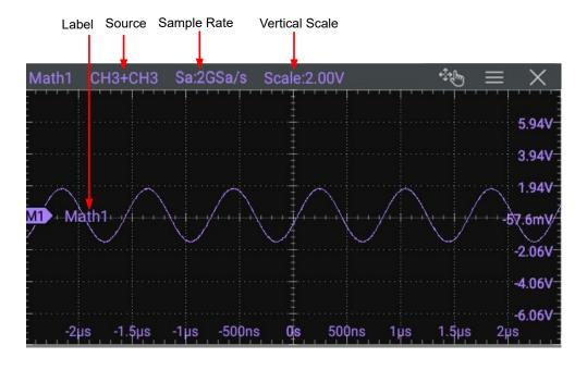
**Figure 9.4 Operation Result Display Window**
