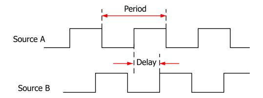
Figure 10.2 Delay and Phase Parameters
