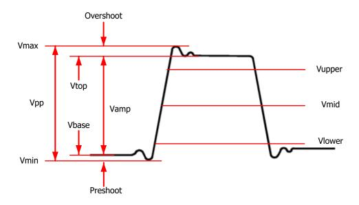
**Figure 10.3 Voltage Parameters**
