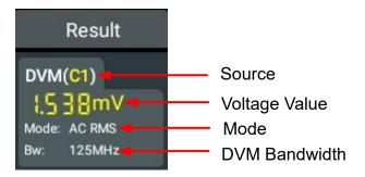
The voltage value in the label shows the measurement extrema over the last 3 seconds.
