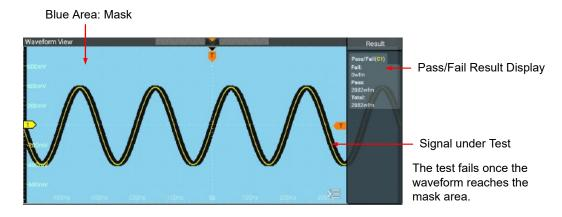
Figure 14.3 Pass/Fail Test Interface
