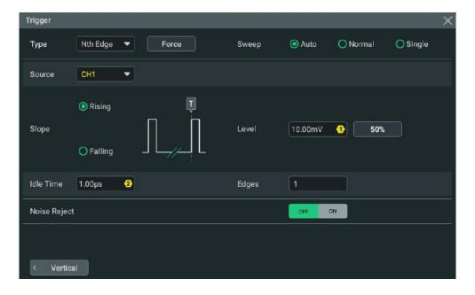
Figure 8.23 Nth Edge Trigger Setting Menu
