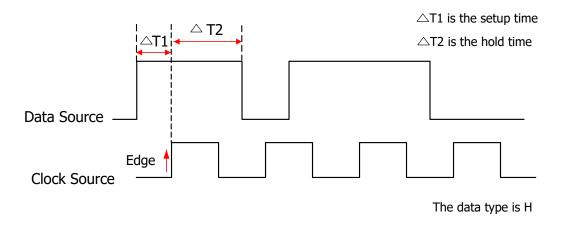
Figure 8.20 Setup/Hold Trigger
