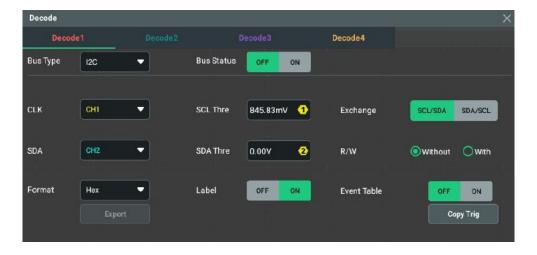
Figure 15.8 I2C Decoding Menu
