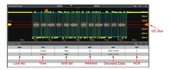
Figure 15.9 I2C Decoding Event Table
