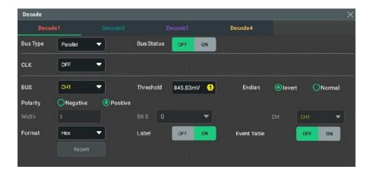
**Figure 15.2 Parallel Decoding Menu**
