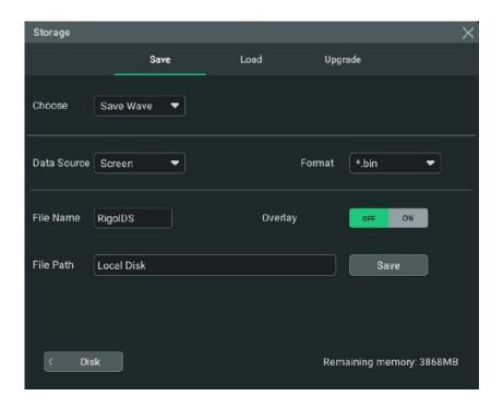
**Figure 20.2 Waveform Saving Setting Menu**
