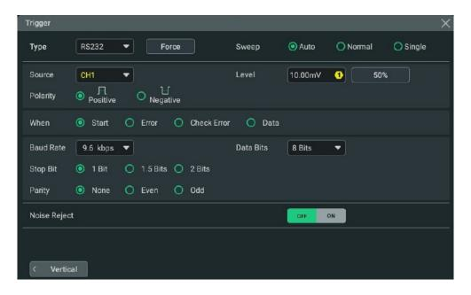
Figure 8.25 RS232 Trigger Setting Menu
