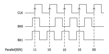
Figure 15.1 Schematic Diagram of Parallel Decoding
