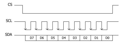
Figure 8.30 Sequential Chart of SPI Bus
