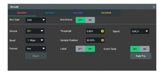
Figure 15.13 CAN Decoding Menu
