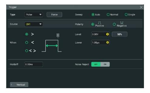
Figure 8.5 Pulse Width Trigger Setting Menu
