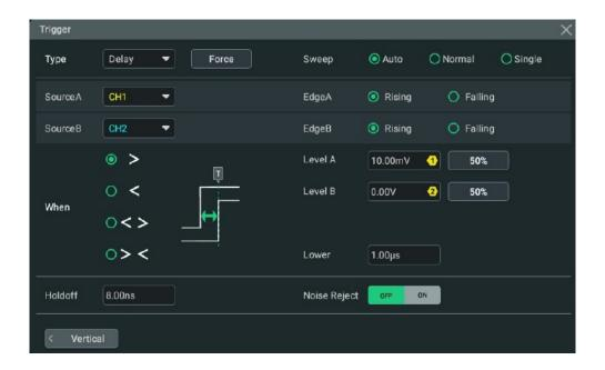
Figure 8.19 Delay Trigger Setting Menu
