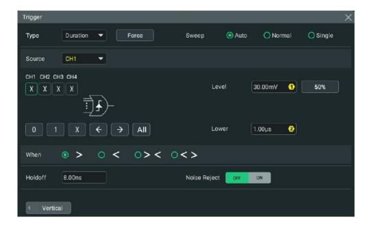
Figure 8.12 Duration Trigger Setting Menu
