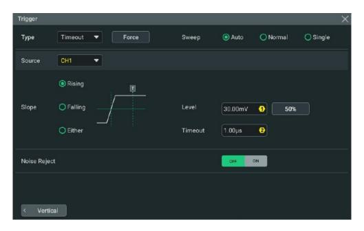
Figure 8.14 Timeout Trigger Menu
