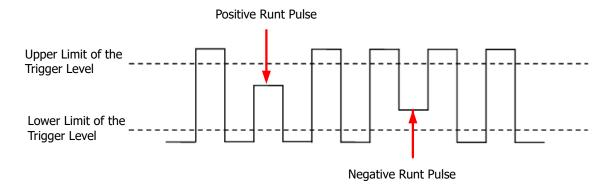
Figure 8.15 Runt Trigger
