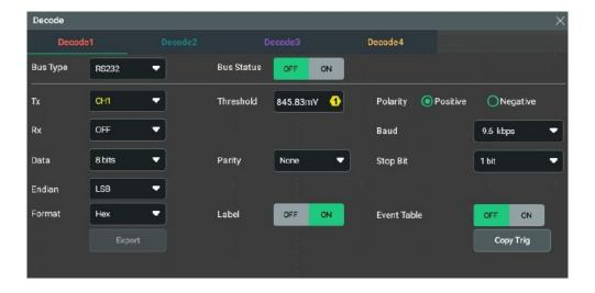
Figure 15.5 RS232 Decoding Menu
