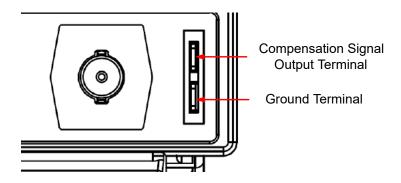
Figure 4.6 Using the Compensation Signal
