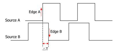
Figure 8.18 Delay Trigger
