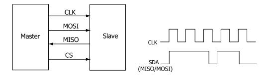
Figure 15.10 SPI Serial Bus
