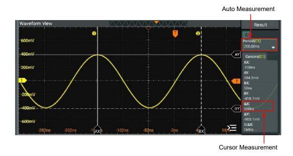
Figure 10.10 Manual Cursor Measurement Example
