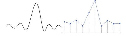
• **Waveform Aliasing:** Aliasing occurs when the sample rate is twice lower than the actual signal frequency (Nyquist Frequency). The frequency of the waveform reconstructed from the sample data is smaller than the actual signal frequency.
