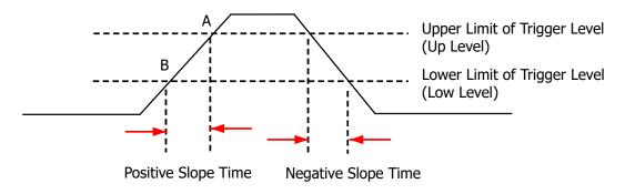
**Figure 8.6 Positive Slope Time/Negative Slope Time**
