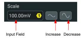
In the **Vertical** menu, click or tap the **Fine** on/off switch to toggle between **ON** (fine adjustment) and **OFF** (coarse adjustment). The default setting is OFF. You can also
