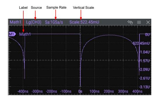
**Figure 9.6 Operation Result Display Window**
