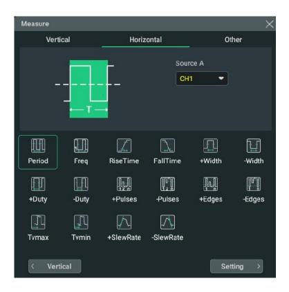
**Figure 10.5 Horizontal Measurement Items**
