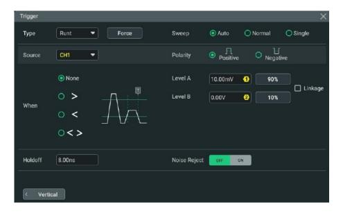
Figure 8.16 Runt Trigger Setting Menu
