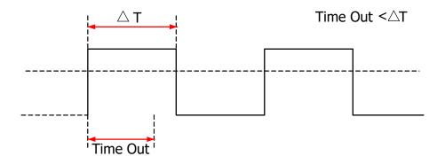
Figure 8.13 Timeout Trigger
