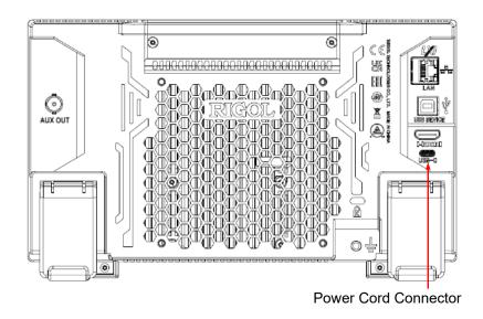
Figure 4.4 To Connect to Power
