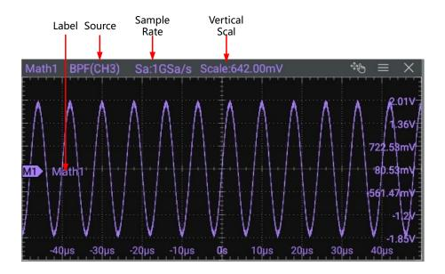
Figure 9.13 Operation Result Display Window
