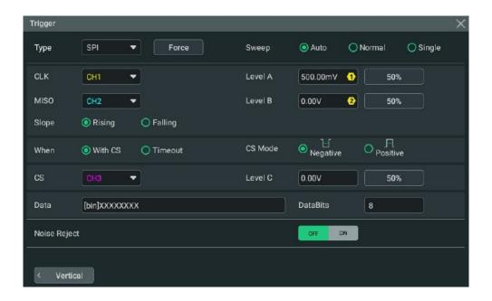
Figure 8.31 SPI Trigger Setting Menu
