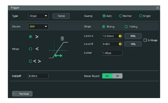
**Figure 8.7 Slope Trigger Setting Menu**
