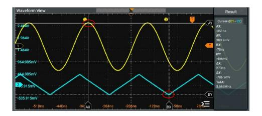
Figure 10.13 Track Measurement (after Horizontal Expansion)
