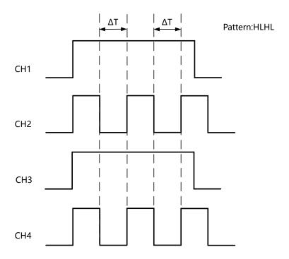
**Figure 8.11 Duration Trigger**
