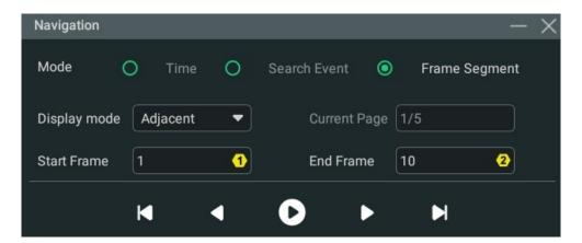
Figure 18.6 "Frame Segment" Navigation Setting Menu
