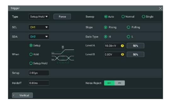
Figure 8.21 Setup/Hold Trigger Setting Menu
