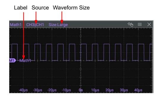
**Figure 9.11 Operation Result Display Window**
