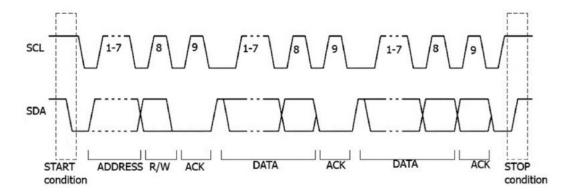
**Figure 8.26 Sequence Diagram of I2C Protocol**
