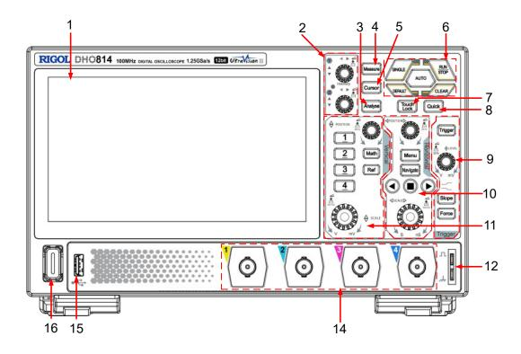
Figure 4.10 Front Panel (4-channel Model)
