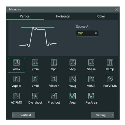
**Figure 10.4 Vertical Measurement Items**
