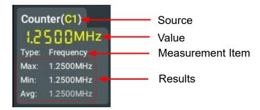
You can click or tap the "Counter" label in the "Result" bar and select **Reset Stat.**, **Setting**, or **Remove** in the displayed window.
