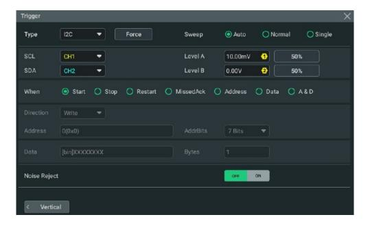
Figure 8.27 I2C Trigger Setting Menu
