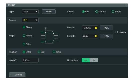
Figure 8.17 Window Trigger Setting Menu
